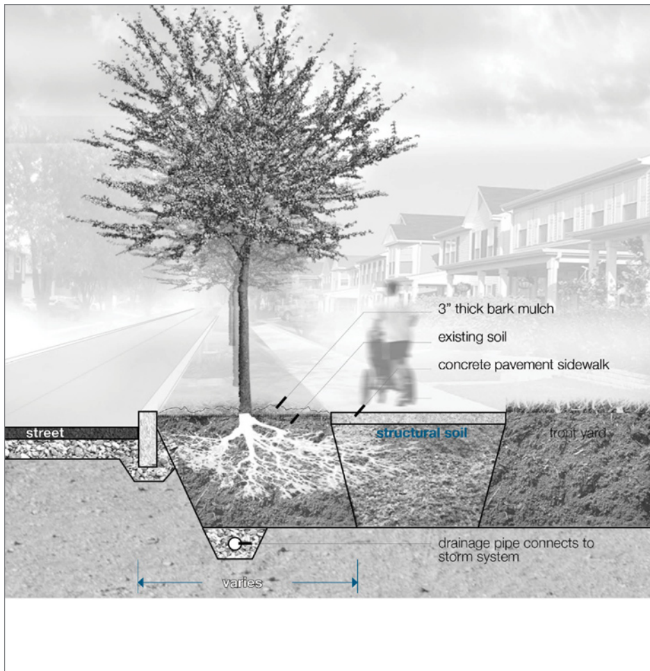
FIGURE 5-33: Cross section of typical tree installation into structural soil under a concrete sidewalk. Note where the tree pit is open, topsoil should be placed around the tree ball, but structural soil can be placed under the ball to prevent tree ball subsidence.
