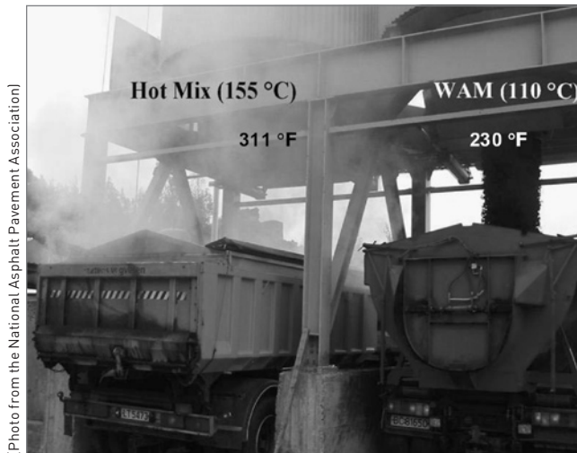
FIGURE 6-3: Reducing the temperature at which asphalt pavement is placed can reduce emissions and energy use. A side-by-side comparison of two trucks shows reduced emissions from cooler mix temperatures.
