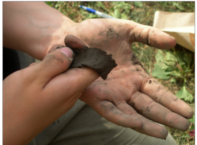
FIGURE 5-10: To form the “ribbon” for texture-by-feel, gently push the soil over the index finger with the thumb. A well-kneaded sample facilitates forming the ribbon.
