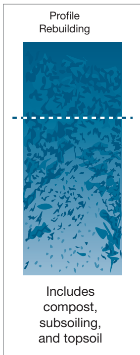
FIGURE 5-25: Schematic of reconstructed soil profile. Note that the incorporation of organic matter at depth creates veins of compost that prevents soil from recompacting and allows root penetration.
