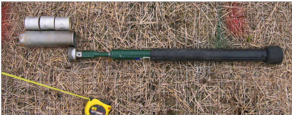
FIGURE 5-17: A soil slide hammer showing three sample sleeves next to the core sampler.
