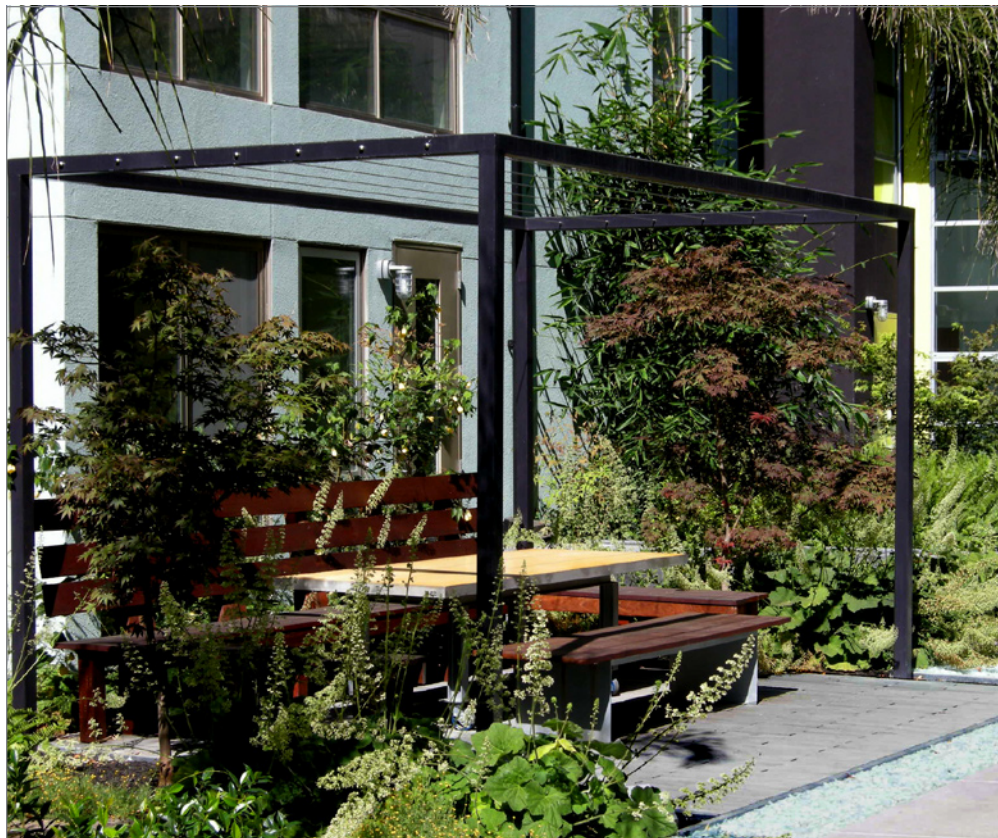
FIGURE 6-34: Wood for the benches in the Dining Arbor at the Pacific Cannery Lofts in Oakland, California, is FSC-certified Ipe, a very decay-resistant Brazilian hardwood.
