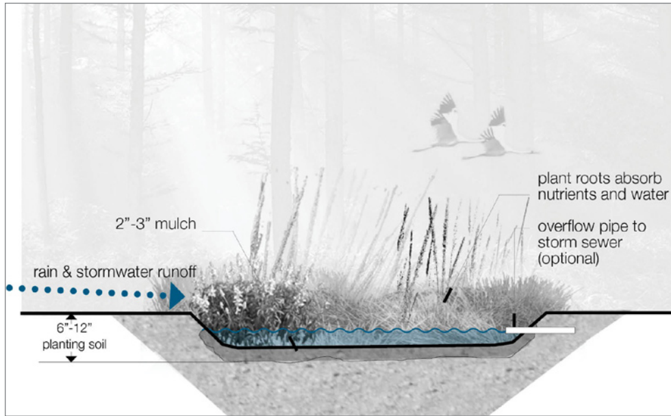
FIGURE 3-34: Typical rain pocket in a residential application.
