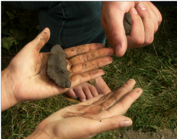
FIGURE 5-9: A kneaded clump of moistened soil ready for analysis by texture-by-feel.
