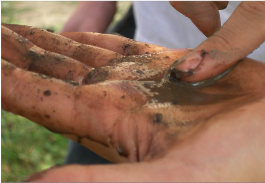
FIGURE 5-12: Rubbing excessively wet soil in the palm of the hand is the final step of the texture-by-feel analysis.
