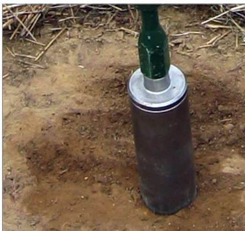
FIGURE 5-18: Once the sample sleeves are fitted inside the core sampler, it is mounted on the hammer and positioned over the area to be sampled. After the soil core is extracted, the center sample sleeve is trimmed with a knife to create an undisturbed sample of a known volume. Some core samplers will only take two sleeves; in that case, the bottom sleeve may be used to prevent compaction by the hammer.
