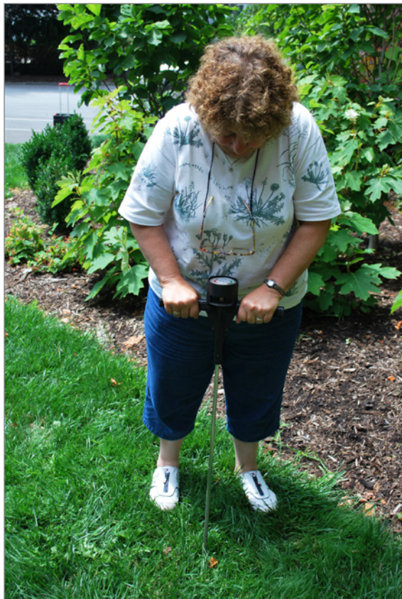
FIGURE 5-16: An inexpensive soil cone penetrometer. Wider cone tips are fitted on the rod for softer soils.
