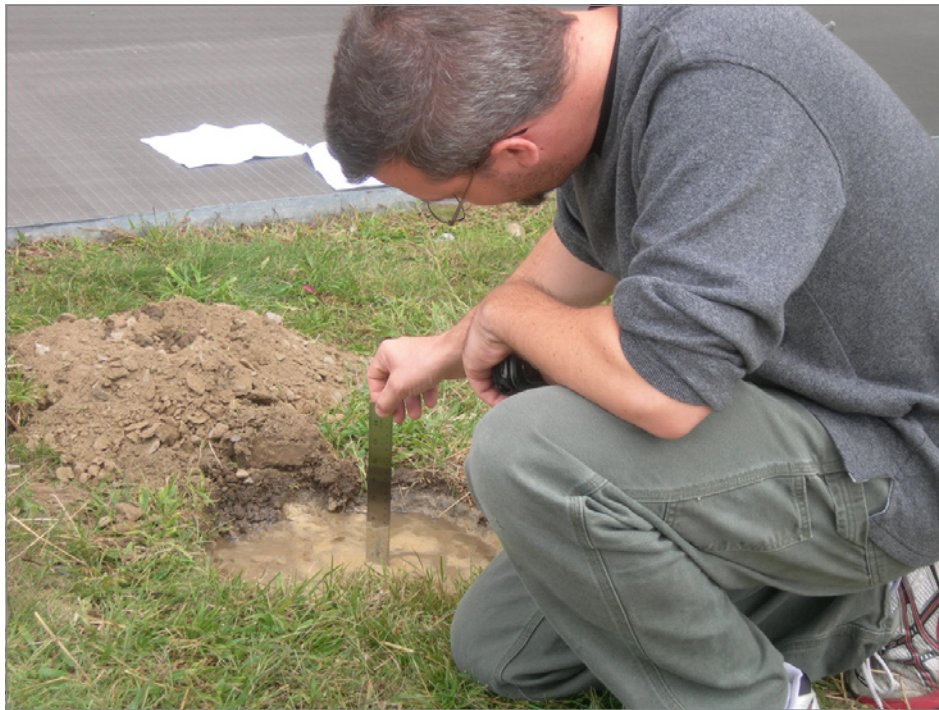
FIGURE 5-21: A simple perc test provides a rapid estimation of internal soil drainage.
