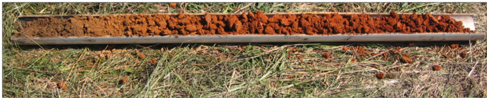
FIGURE 5-4: A soil profile excavated with an auger and laid out in a tray. Note the typical color and structure progression from left to right [surface to subsoil] of this Shottower loam soil that has been under agricultural production for many years.
