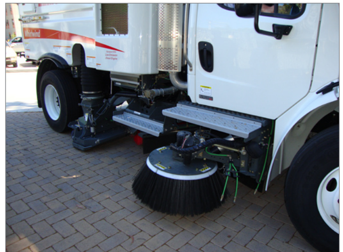
FIGURE 8-19: Vacuum sweepers should be used several times a year to clear debris and clogging from porous pavements.
