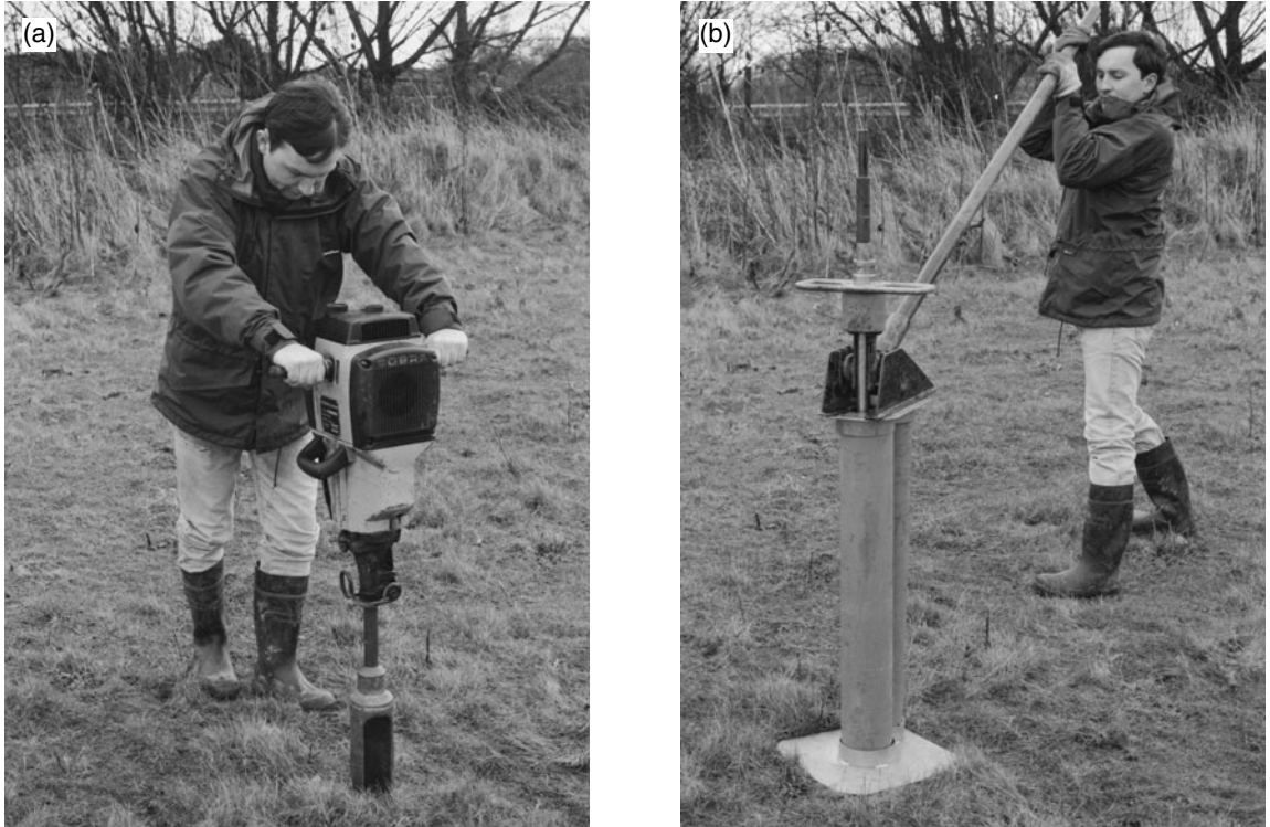
FIGURE 2.10 Small scale mechanical auger system for soil and sediment study: (a) drilling in a window sampler, (b) levering it out.
