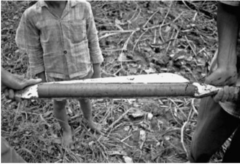
FIGURE 3.32 Borehole core sampling using manual equipment.
