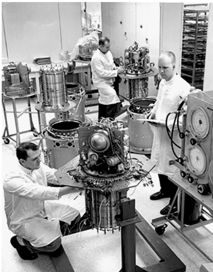
Figure 16 Pratt & Whitney technicians assemble alkali fuel cells for Apollo service modules, 1964. (From Ref. 43.)
