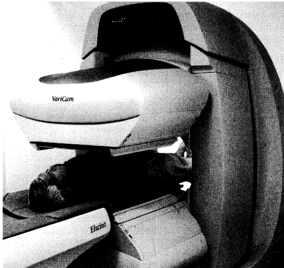
FIG. 12-28 Dual head gamma camera is capable of single photon emission computed tomography (SPECT) imaging and simultaneous posterior whole body and planar imaging.
