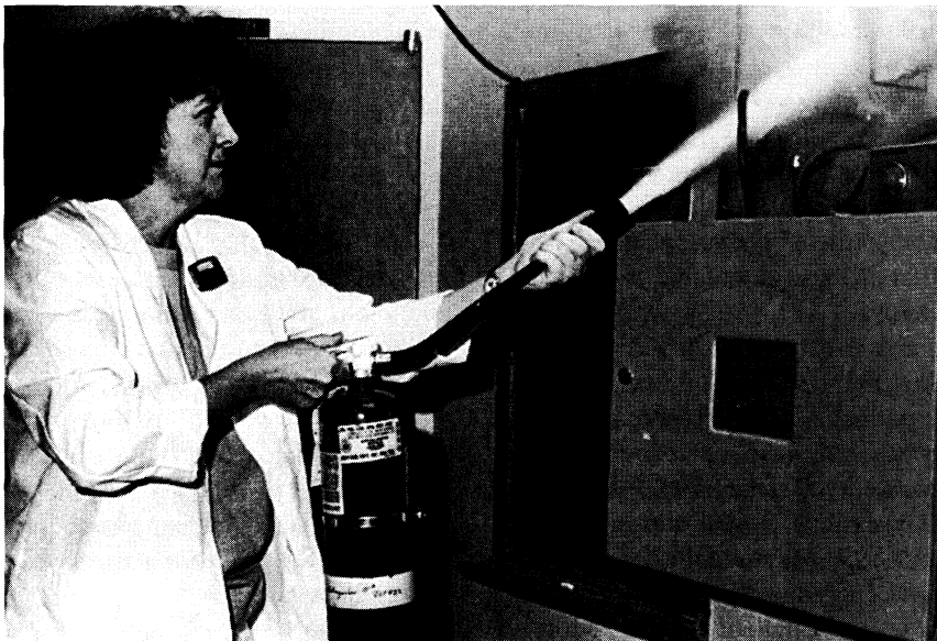
FIG. 4-5 Use fire extinguisher in a sweeping motion from side to side at the base of the flame. Stand back at a safe distance.
