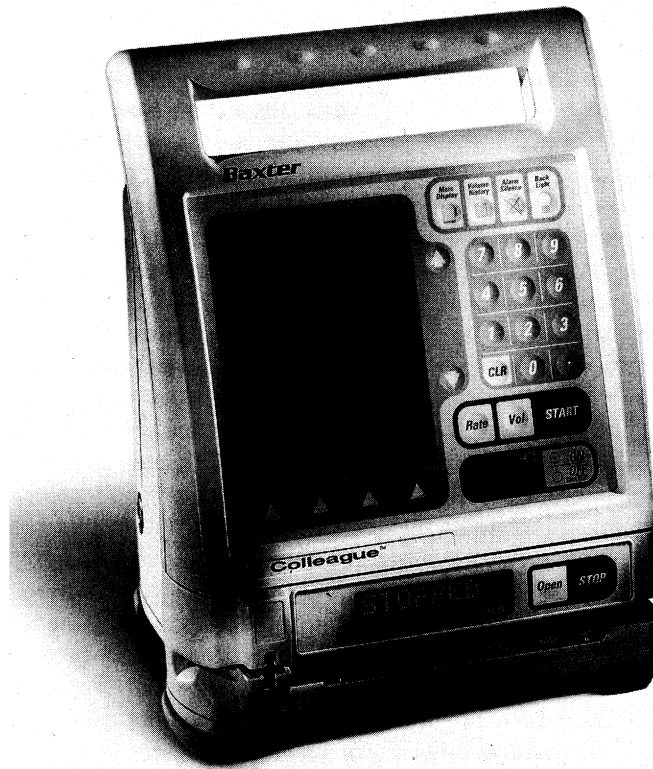
FIG. 7-17 IV pumps regulate infusions and permit self-administration of IV medications.
