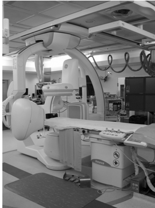
FIGURE 11.3. The GE Innova biplane angiography suite at the authors' facility provides images in two planes at the same time, thus allowing better visualization, fewer injections of contrast, and shorter procedure time. The technology features rotational angiography and 3D reconstruction, and it is also capable of producing cross-sectional images like a computed tomography (CT) scan. The neuroanesthesiologist and the ventilation machine are best located to the patient's left side given the confines of the angiography apparatus.
