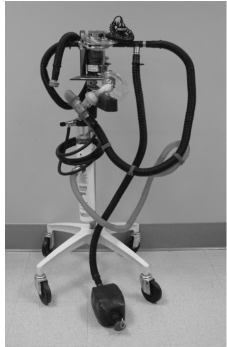
FIGURE 28.5. Gegel-Mercado Modification to the Ohmeda U-PAC. Note the increased length of reservoir tubing on the inspiratory end, or left, of the vaporizer. This configuration is equipped with an oxygen analyzer and scavenging apparatus (termination of light blue tubing, extending from face mask). It can be further configured to accommodate gas sampling and spirometry. (Photo by Clinkscales CP, 2009.)
