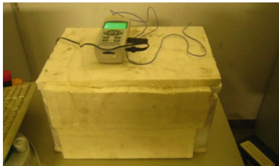
Fig. 5.11 Temperature measurement inside insulated mould
