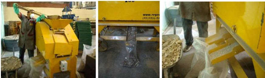
Fig. 4.19 Grinding process with crusher
