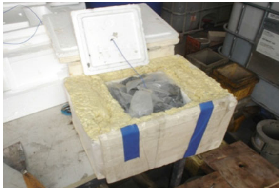
Fig. 5.10 Insulated mould inducing semi-adiabatic boundary conditions on the curing concrete sample
