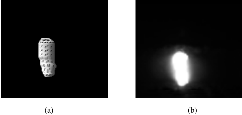
Fig. 1. The visualization model of MCBs switching arc(a) and the image gathered(b)
