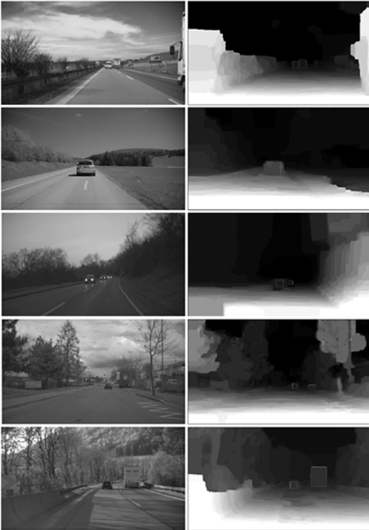
Fig. 8. Examples of manually specified rectangular regions for approximated ground truth: in original sequences of Set 1 on [4] (left) and in Sobel-based BP results (right)
