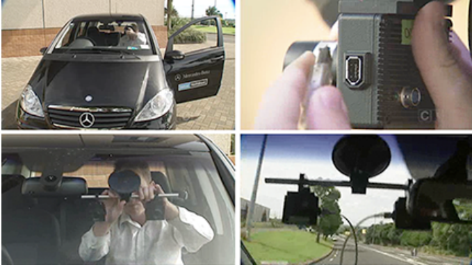
Fig. 7. Test vehicle HAKA1 with a pair of cameras for stereo image sequence capture, recording stereo sequences on Auckland’s roads since July 2008
