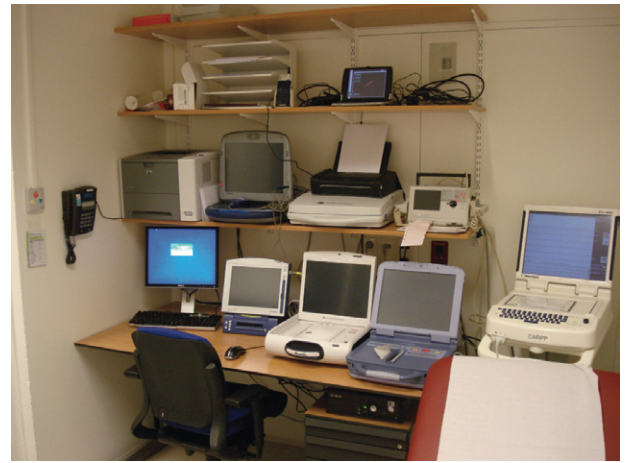
FIGURE 37-5 Dedicated pacemaker follow-up room with a variety of programmers. This picture shows how a dedicated pacemaker follow-up room can be arranged. Some essential equipment can be seen: emergency alarm system and telephone, computer and printer facilities connected to the Internet, multiple programmers of different pacemaker manufacturers, defibrillator, fitted with external pacing capabilities, ECG recording system, and patient examination table.
