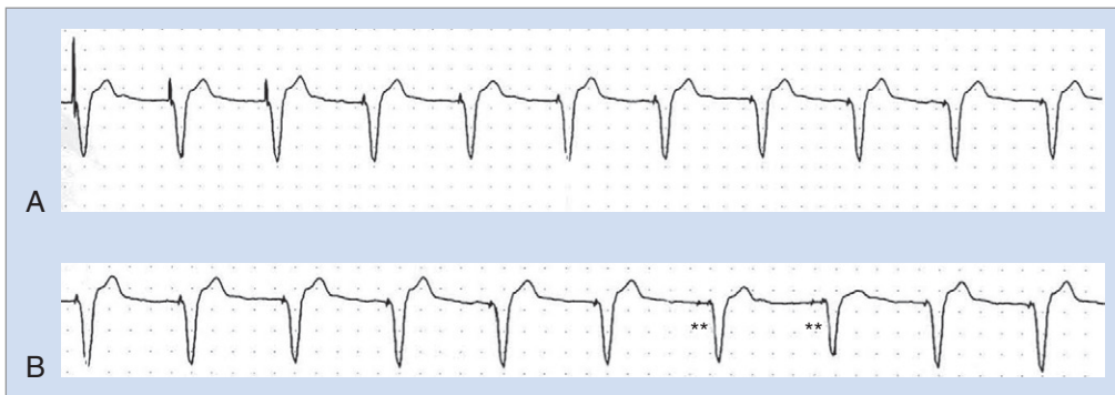
FIGURE 36-11 A and B , Continuous rhythm strip demonstrating the AutoCapture algorithm with Beat-by-Beat Capture Confirmation (St. Jude Medical, Little Canada, MN) in action. This is a threshold-tracking algorithm that confirms beat-by-beat capture of each pacemaker stimulation. It initially starts with a high energy output at the start of A . Automatic capture verification monitors every beat for the presence of an evoked response. Automatic reduction in energy output occurs, as seen in A , with gradual reduction in the height of the pacing stimulus. Loss of capture seen in B in the areas marked by asterisks triggers an automatic backup safety pulse (two closely spaced pacing spikes) to ensure capture in the absence of an evoked response. The automatic output regulation sets the output just above the measured threshold in the next two beats. This feature ensures the lowest energy output required for capture and helps optimize device longevity.
