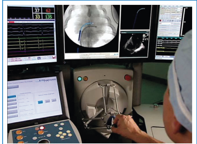
FIGURE 16-10 Composite photo of the Sensai system remote robotic navigation. (Courtesy Hansen Medical, Mountain View, CA.)
