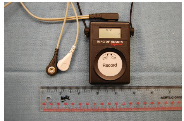
FIGURE 69-3 An example of a looping event recorder. In order to store electrograms preceding the event, the patient wears electrodes continuously during the monitoring period.
