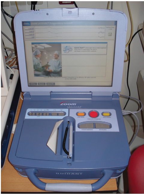
FIGURE 379-4 Combined pacemaker and implantable cardioverter defibrillator (ICD) programmer from Boston Scientific Corp. On a programmer device, the following generic key components can be seen: telemetry wand for wireless contact with the pacemaker, electrocardiogram cable, touch screen with pencil, buttons for emergency therapy and to abort therapy, buttons for interrogation and (re)programming, and paper strip printer with print buttons.
