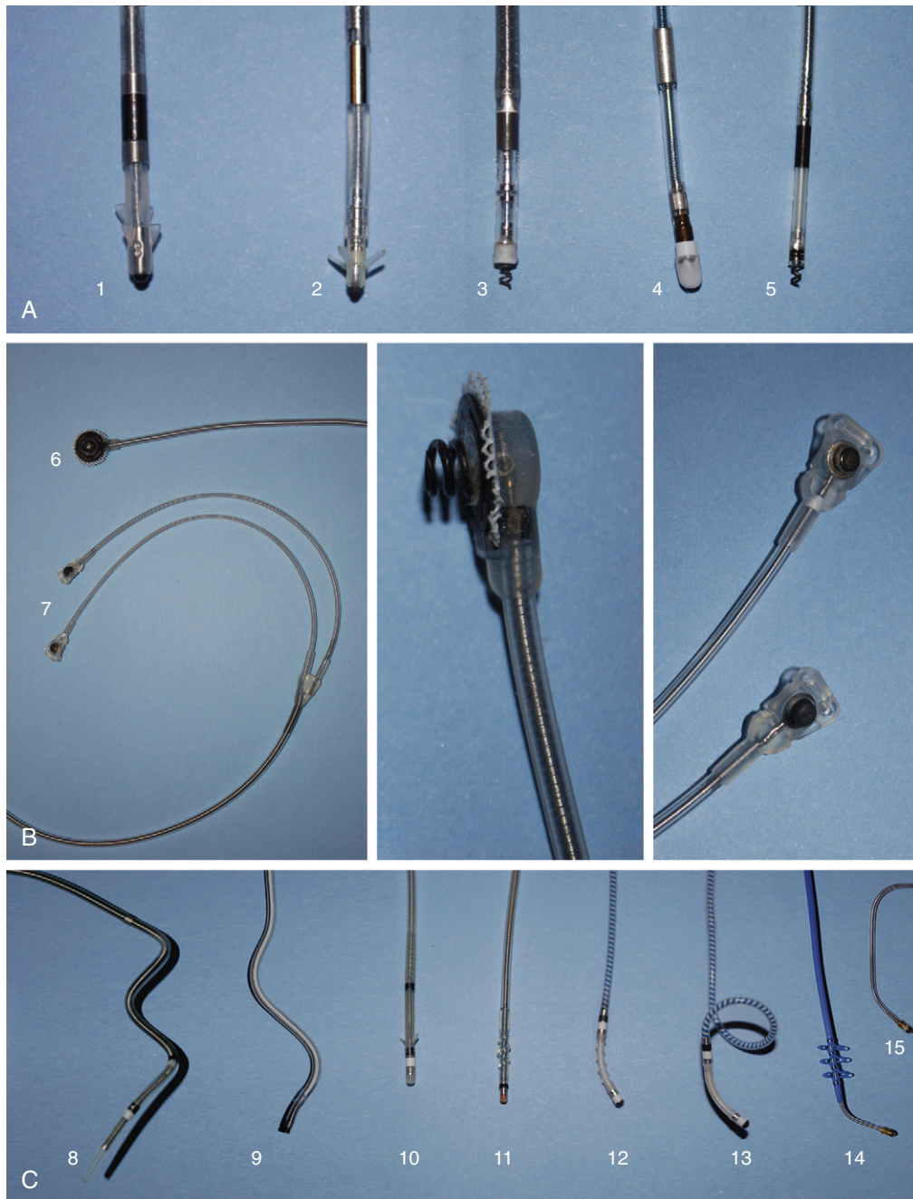
FIGURE 37-3 Pacemaker electrodes. A , Straight endocardial passive fixation (tined) electrodes (1, 2) and active fixation (screw-in) electrodes (3, 4, 5). One (nonretractable) screw-in lead is covered with a dissolvable coating (4). B , Epicardial bipolar electrodes. Screw-in electrode (6) and suture-on electrode (7). Middle , Close-up (side view) of a screw-in electrode (6). Right , close-up of a suture-on electrode (7). C , A variety of passive fixation coronary sinus electrodes. Fixation can be achieved by wedging the preshaped distal tip of the electrodes (8, 9, 13, 15) or the small silicone fins or lobes (10, 11, 12) into the vein. Electrode 14 shows an electrode that combines a preshaped tip with deployable lobes.
