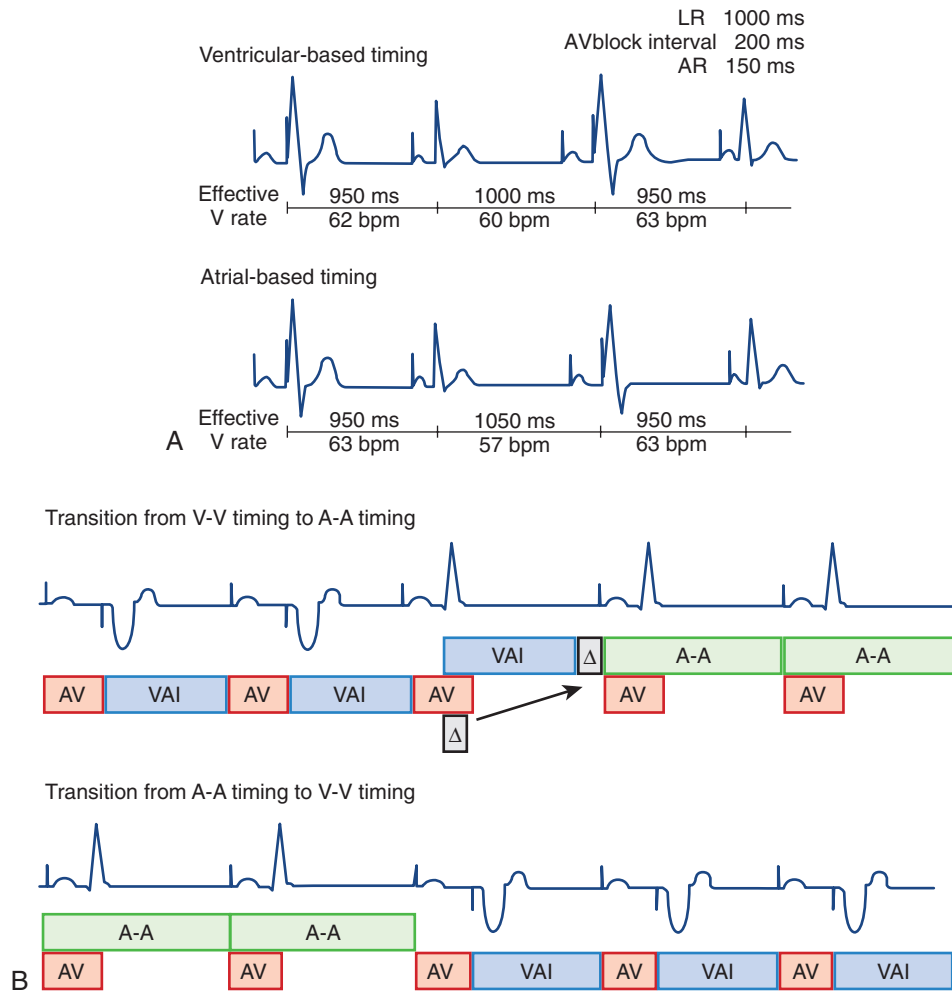
FIGURE 34-6 Atrial, ventricular, and hybrid base-rate behavior. A , Ventricular and atrial-based timing with underlying 2:1 atrioventricular (AV) block (AV block interval is longer than atrial rate). Top : AV block interval is slightly longer than atrial rate, hence the rate alternates with the rate at the lower rate limit (LRL; 60 beats/min) and slightly faster than the LRL (63 beats/min) in ventricular-based timing. Bottom : Atrial-based timing violates LRL with an alternating faster (63 beats/min) and slower (57 beats/min) ventricular rate than programmed LRL. B , Hybrid-based timing. 6 Top : Timing changes from ventricular based to atrial based after a ventricular sensed event is noted ( \Delta , difference between P-R interval and A-V interval in the first cycle during which intrinsic conduction occurs). \Delta is applied to next V-A interval (VAI) to provide a smooth transition without affecting V-V intervals. Bottom : Timing changes from atrial based to ventricular based when intrinsic AV nodal conduction is no longer present. ( A , From Ellenbogen KA, Wood MA: Cardiac pacing and ICDs, ed 4, Malden, MA, 2005, Blackwell; and Siemens-pacesetter; B , From Insignia I Ultra System Guide, models 1190/1290/1291, St. Paul, MN, 2006, Guidant Corporation.)
