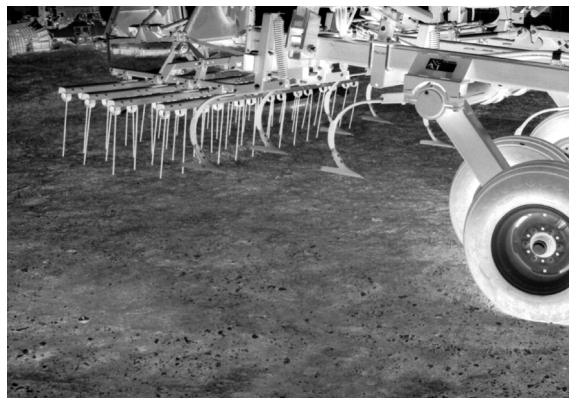
Figure 7.5 Cultivator. Arrow-shaped tillers followed by harrow teeth are moved between the crop rows to destroy the weeds.
