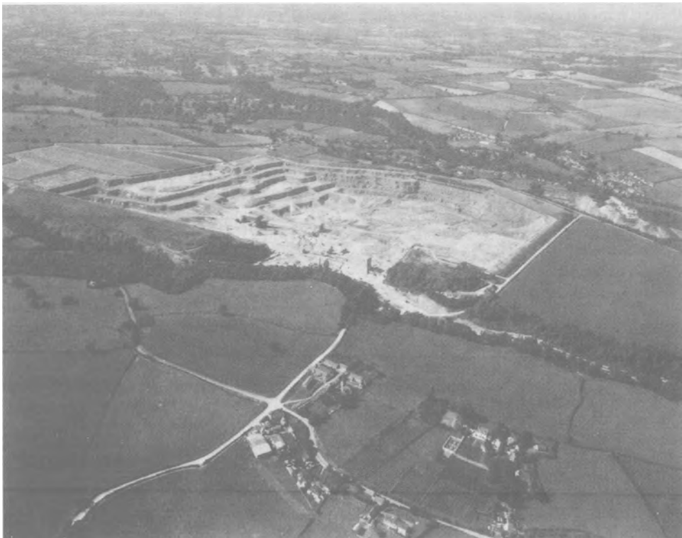
FIG. 4.2. Large limestone quarry showing benches, process plant, rail and road access (courtesy of ARC Ltd).
