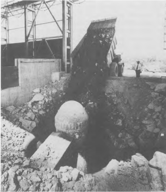
FIG. 5.3. Dump truck discharging into a primary gyratory crusher (courtesy Nordberg (UK) Ltd).
