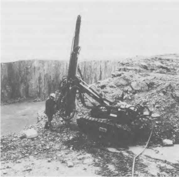
FIG. 4.11. Crawler mounted DTH drill (courtesy of Halco Ltd).
