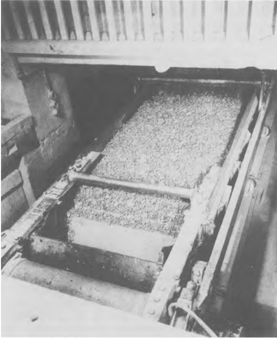
FIG. 5.25. Horizontal vibrating (resonance) screen (courtesy Nordberg (UK) Ltd).
