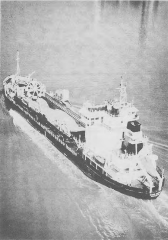
FIG. 4.22. Dredger with bucket wheel discharge (courtesy of RMC Ltd).
