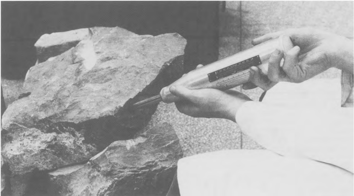
FIG. 7.14. Schmidt concrete test hammer.
