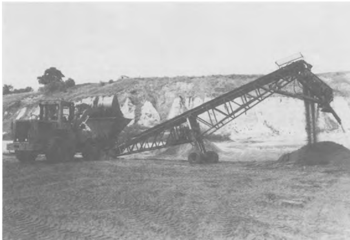
FIG. 9.9. Typical dry screening operation in UK sand quarry.
