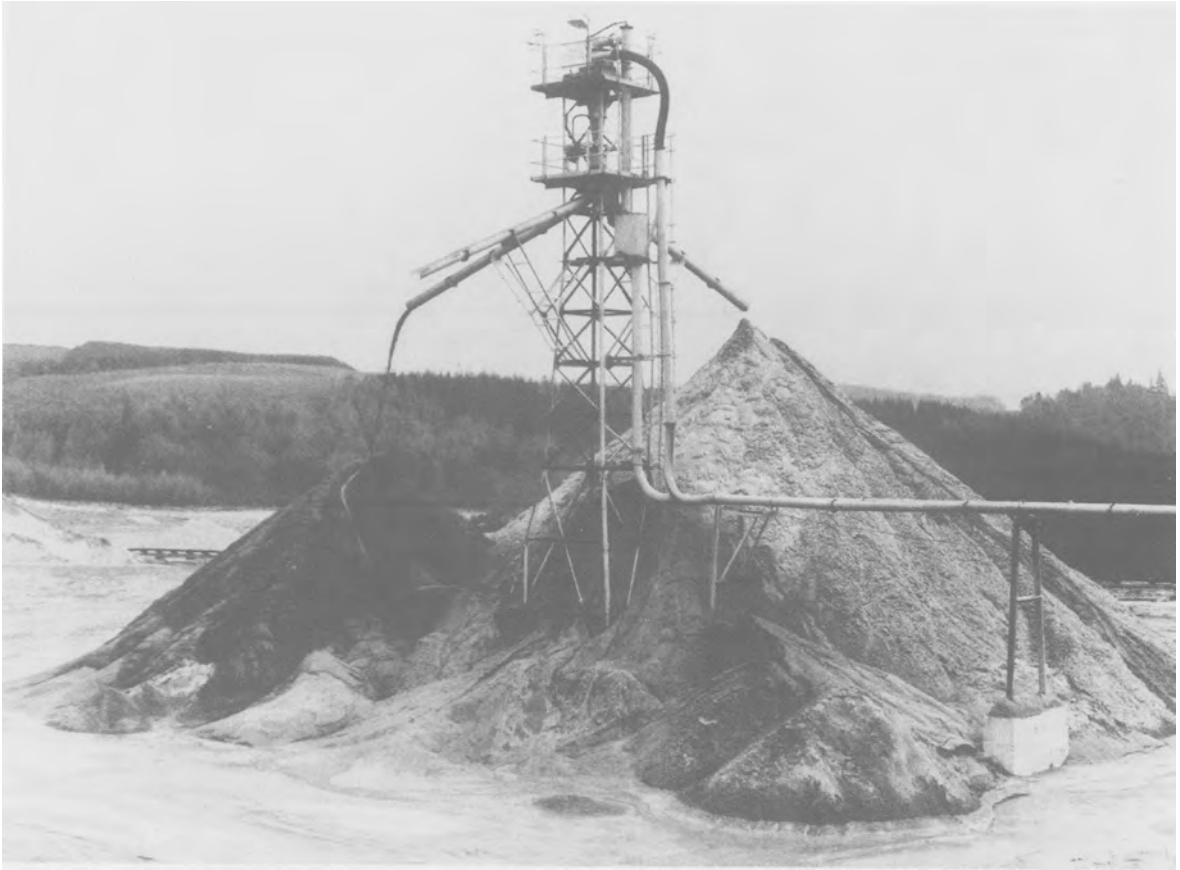
FIG. 5.44. Hydrocyclone mounted in a tower (courtesy Linatex Ltd).
