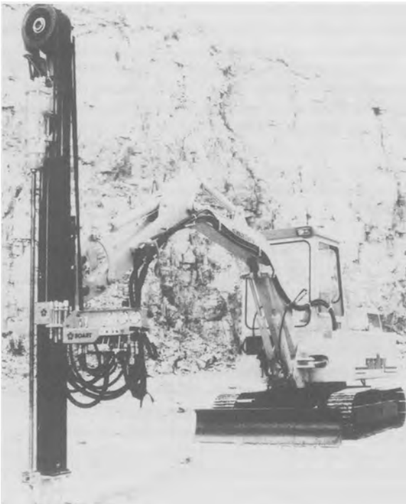
FIG. 4.12. Small diameter, top hammer (drifter) drill mounted upon articulated arm (courtesy of Boart).
