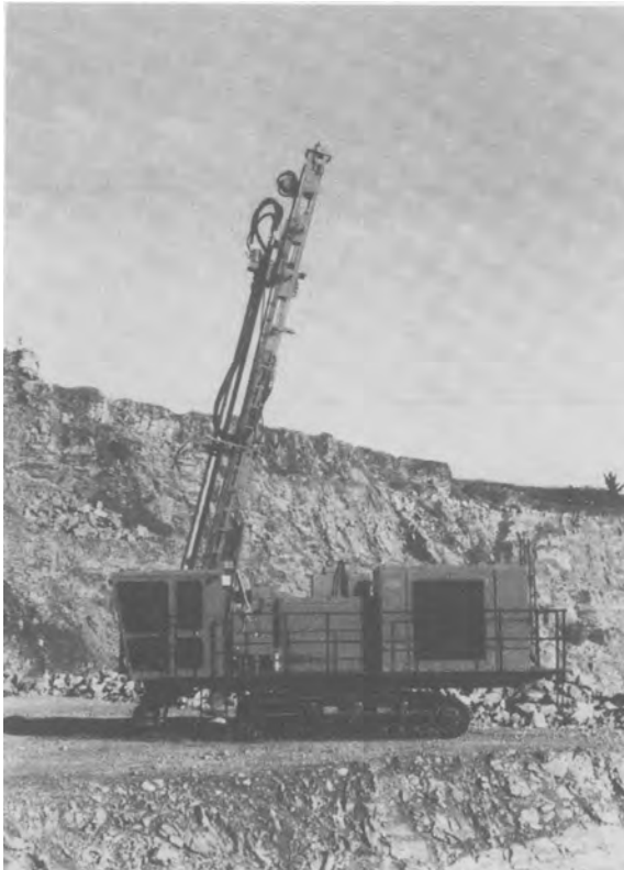
FIG. 4.9. Large pneumatic (DTH) blast hole drill (courtesy of ARC Ltd).
