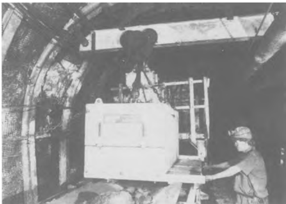
FIG. 5.41. Suspended magnet collecting tramp metal (courtesy Boxmag-Rapid Ltd).
