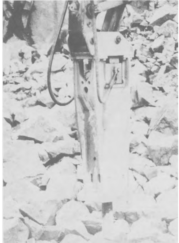
FIG. 4.15. Hydraulic hammer (courtesy of Krupp).
