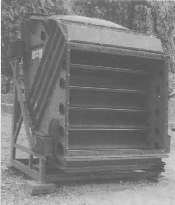
FIG. 5.29. Mogensen probability screen (sizer) (courtesy Mogensen Sizers Ltd).
