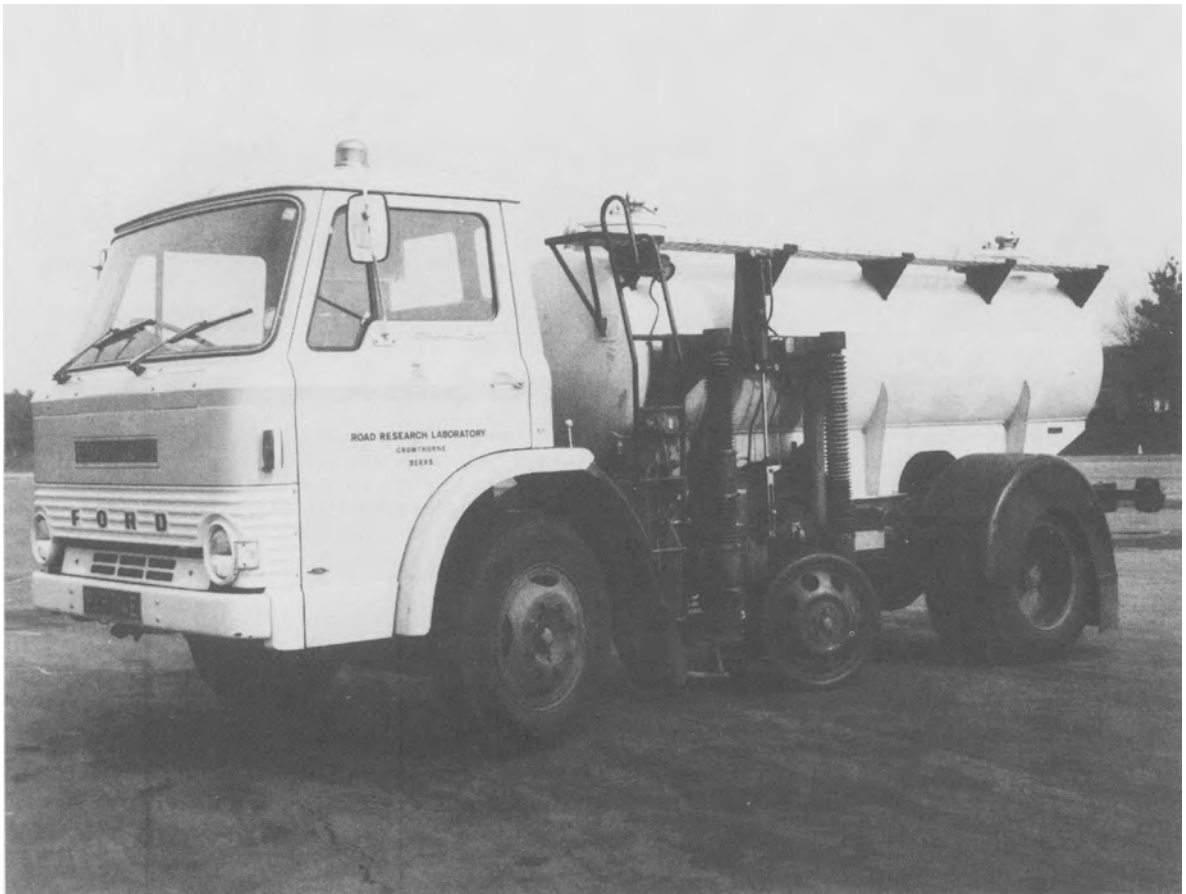
FIG. 11.4. Sideway force coefficient routine investigation machine (SCRIM) used to monitor the skidding resistance of in-service roads (Transport and Road Research Laboratory).
