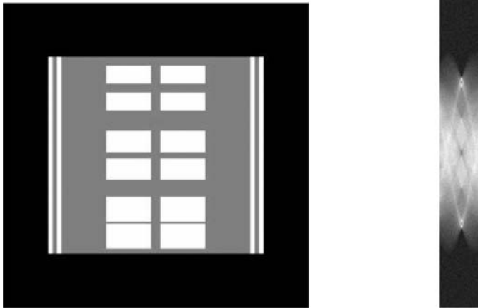
FIGURE 1. A 341 \times 341 pixel representation of a 2D image (left) and its 1D projections (right). Each projection consists of noisy versions of line integrals for 495 parallel lines (the distance between them is the same as the length of an edge of a pixel in the image); they correspond to individual columns in the picture on the right. The angle between the lines corresponding to one column and the next one is 2^\circ ; there are 70 columns corresponding to direction angles ranging from -69^\circ to 69^\circ with the vertical. The noise is additive zero-mean Gaussian noise, with a standard deviation that is the integral for a vertical line through the largest of the 12 central rectangular shapes in the image. (The image is approximately a cross-section through a 3D phantom, designed by Fernández et al. (2002), of mitochondria; the just discussed rectangular shapes are sections through the simulated cristae.)
