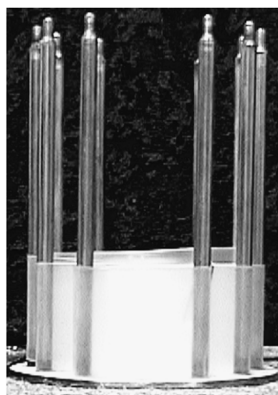
FIGURE 1.4 An example of a SemiPermeable Sampling Device (SPMD).
