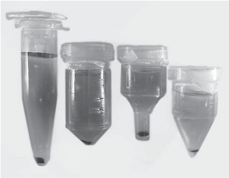
Fig. 2. Tubes for microwave-assisted resin polymerization. Epon resin (recipe 2 from Table 2 ) was used to embed small pieces of mouse liver. The specimens were embedded in resin using tubes of different plastic and shapes. The first tube is a 0.5-mL Eppendorf centrifuge tube. The other tubes are BEEM capsule molds obtained from microscope supply companies.
