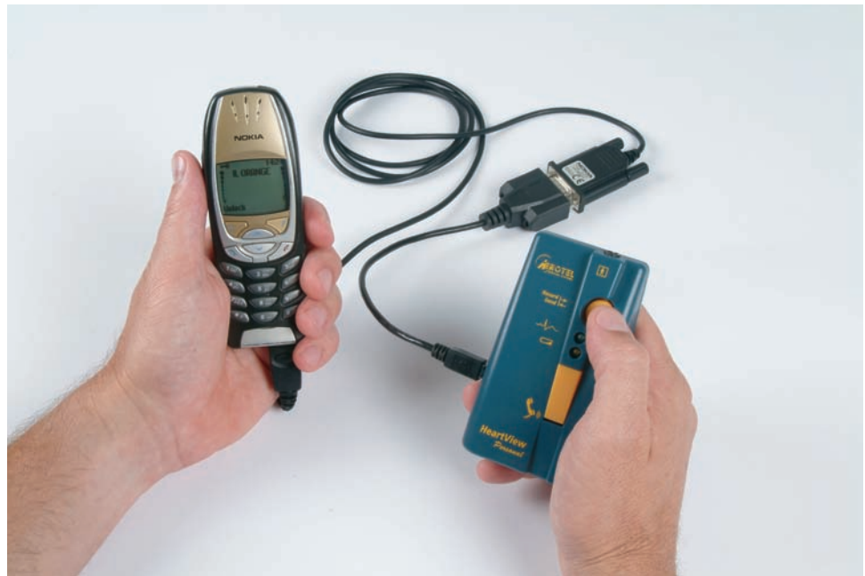
Figure 7-6 Transtelephonic monitors allow information to be transmitted over a phone line or even a cell phone.
