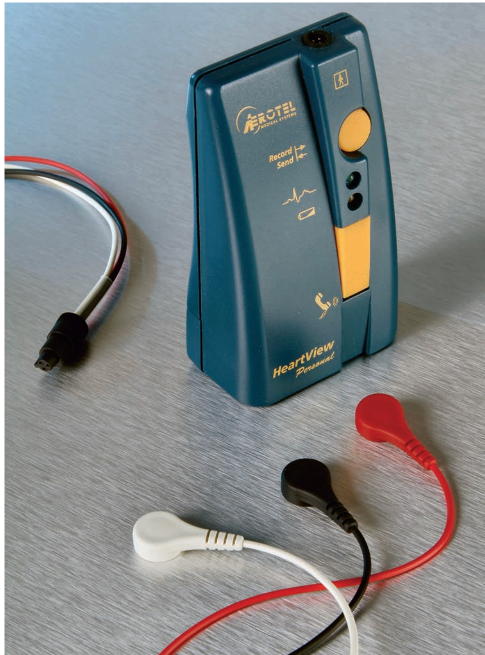
Figure 7-2 Digital ambulatory monitors record the electrical activity of the heart, which can be transferred directly to a computer or over the Internet for interpretation.
