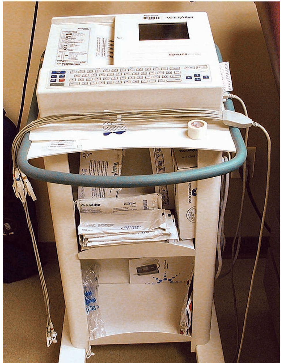
Figure 3-9 A multichannel ECG machine records 3, 4, or 6 leads at a time on a large sheet of ECG graph paper.
