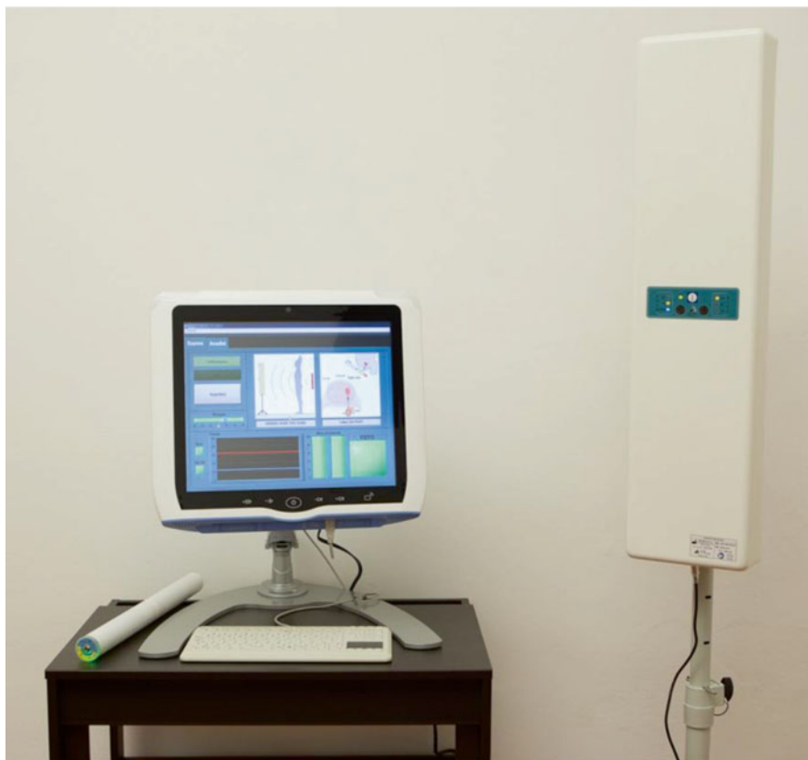
Fig. 6.2 ESO-MED 8G components ( left to right ): probe, diagnostic station, receiver
