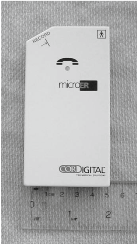
FIGURE 22-2. Transtelephonic monitors. The device is lightweight and portable and is easily placed in a handbag or pocket. Four recording electrodes are present on the back of the device to permit single lead rhythm strip capture. A record button (top left) is pressed in the event of symptoms, and the recorded event is transmitted to a base station over an analog phone line.
