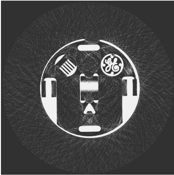
Figure 17.29 Radial artefacts: streak artefacts (very similar to CT) can be seen in the background.
