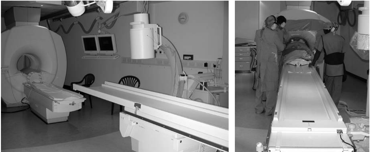
Figure 9.19 Interventional MRI system with integral C-arm X-ray tube over an extended patient couch. This system is used for pediatric cardiac endovascular procedures (courtesy of Dr S Keevil, Guys' Hospital, London).
