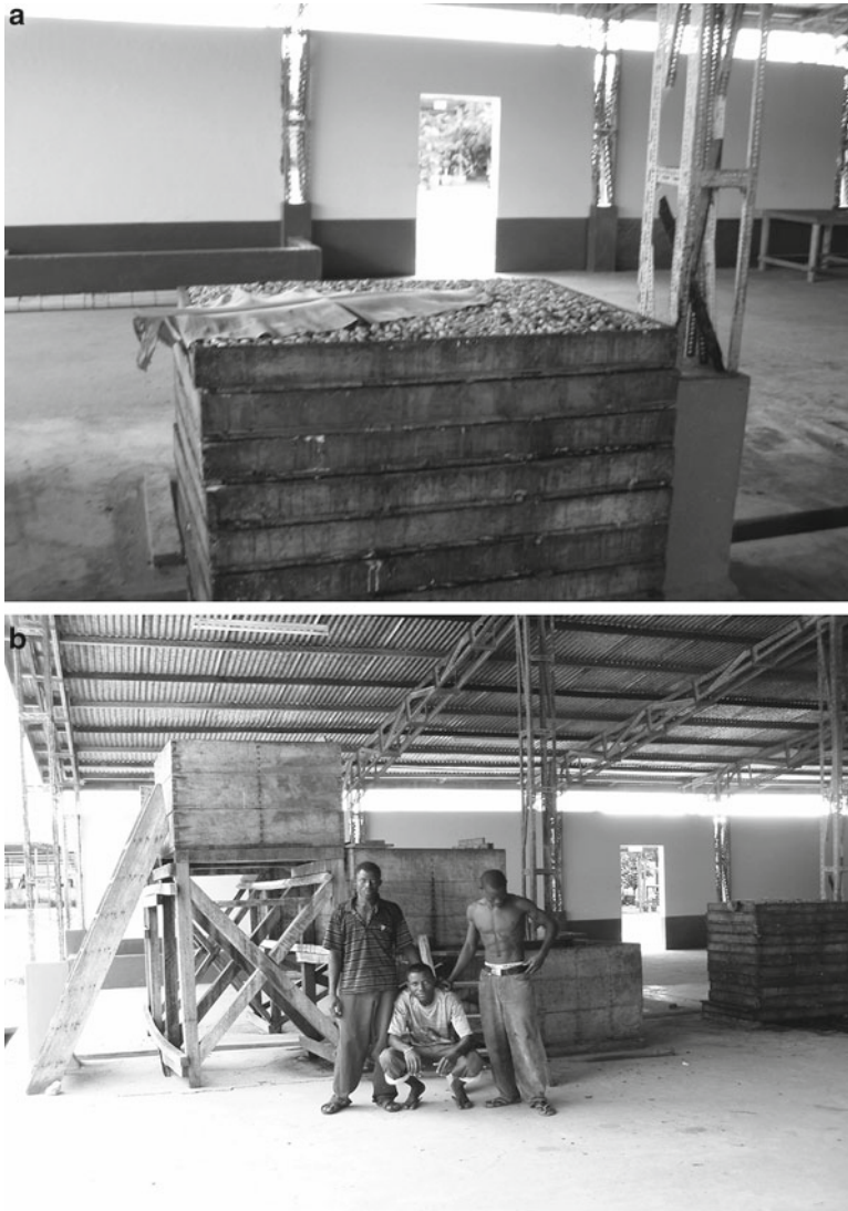
Fig. 4.3 (a) Tray fermentation. (b) Box fermentation of cocoa beans (Pictures courtesy of D.S. Nielsen)
