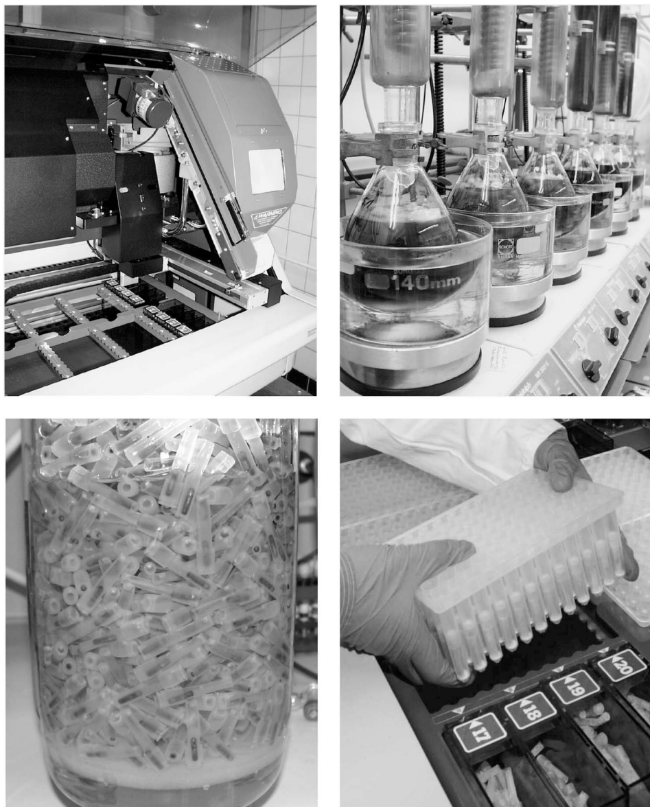
Figure 9.8 Automated directed sorting of micro-reactors (top left). Sets of micro-reactors are reacted with their respective building block in round-bottom flask (top right). Washing of the pooled reactors (bottom left). Micro-reactors arrayed into a cleavage block (bottom right).
