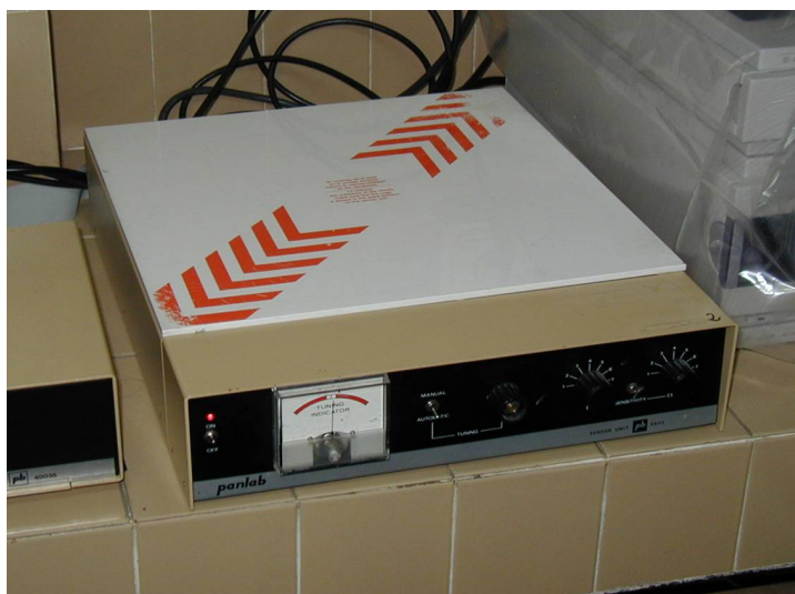
Fig. 3. Complementary tests: Sensor unit of the actimeter. This unit registers the variations of the oscillation frequency in the electromagnetic field produced by the mouse' movements.
