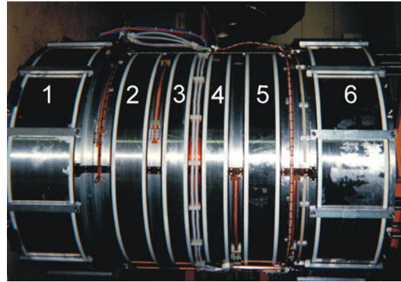
Fig. 12 Coil profile of a 3 T unshielded MRI magnet illustrating typical coil placement. The discrete multiple coils are denote by numbers in the picture
