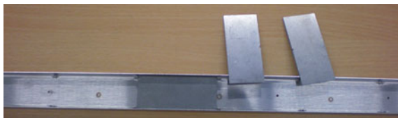
Fig. 18 Set-up for passive shimming a magnet
