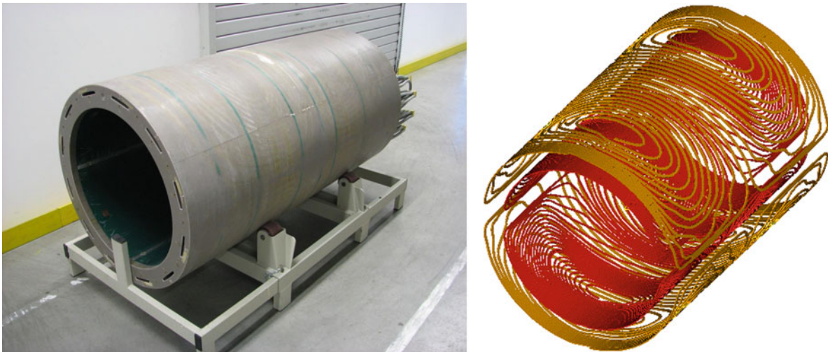
Fig. 1 Left : a gradient coil cylinder potted with resin incorporating the gradient windings. Right : A typical wire path for a transversal gradient—primary layer in red, secondary in orange
