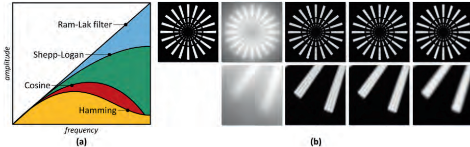
Figure 2.5: (a) Different filters. A ramp function can be used to undo blurring, but is sensitive to noise. Other filters attempt to compensate for higher frequency values. (b) Example of different reconstruction filters. From left to right: original image, non-filtered image from simple back-projection, ramp filter, Shepp-Logan filter, cosine filter. The bottom row shows a magnified region in the lower-left the image, where subtle reconstruction artifacts are removed.
