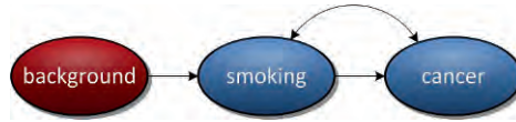
Figure 8.14: A causal graph where P(\text{cancer} \mid \text{do}(\text{smoking})) is not identifiable in general, but is identifiable using linear Gaussian models.
