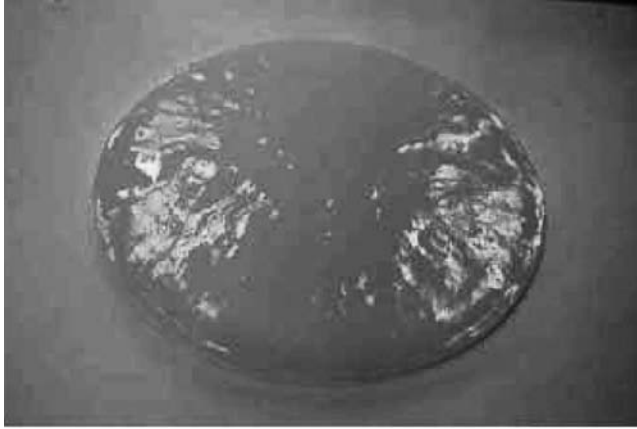
FIGURE 6.2 Bacterial cellulose–chitosan composite in the initial wet state of the never dried sheets.
