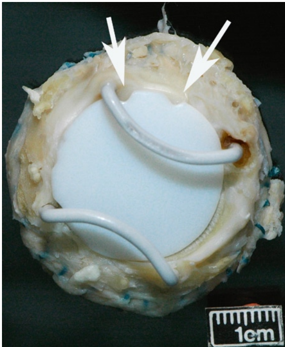
Fig. 11.43 Excised mechanical prosthesis with a plastic disc and struts. Repetitive movement has eroded pieces of the plastic disc where it hits the struts ( arrow )
