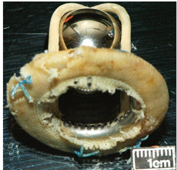
Fig. 11.45 Excised Starr Edwards mechanical prosthesis with cloth wear where the ball hits the ring. The cloth is frayed and irregular “teeth” are exposed. Such patients often have hemolysis
