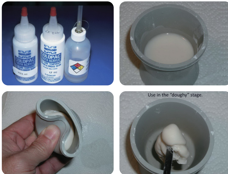
Figure 3.D.4. Motloid ColdPac is mixed in a rubber dappen dish until it reaches a doughy consistency, at which point it can be kneaded with the sides of the dish to further improve the mix.
