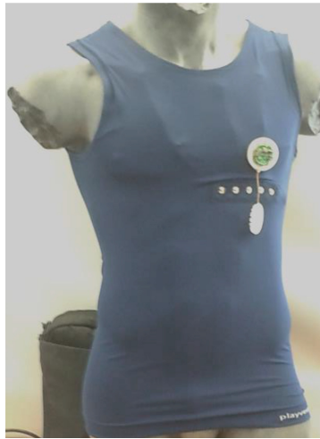
Fig. 3. The SIVIC T-shirt and data acquisition module
