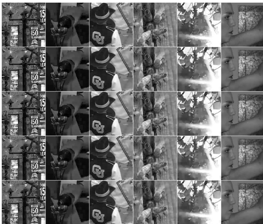
Fig. 4. Frames from sequence 1, 4, 6, 7, 8, 9 (column-wise); Frames: compressed, restored with dictionary of size 256, restored with dictionary 256x8; restored using [8]; restored using the h.264 deblocking alg. (row-wise)
