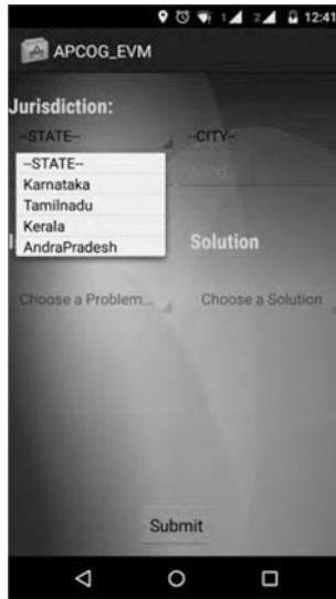
Fig. 1 The mobile application developed for waste management has the main activity consisting of three fields: Jurisdiction , Issue , and Solution . Within the jurisdiction field are two dropdown fields that have 'state,' 'city' as contents. When a state is selected, the corresponding cities are listed. There are two textboxes namely 'area' and 'ward,' in which users need to input the area of the ward where there is a waste management issue
