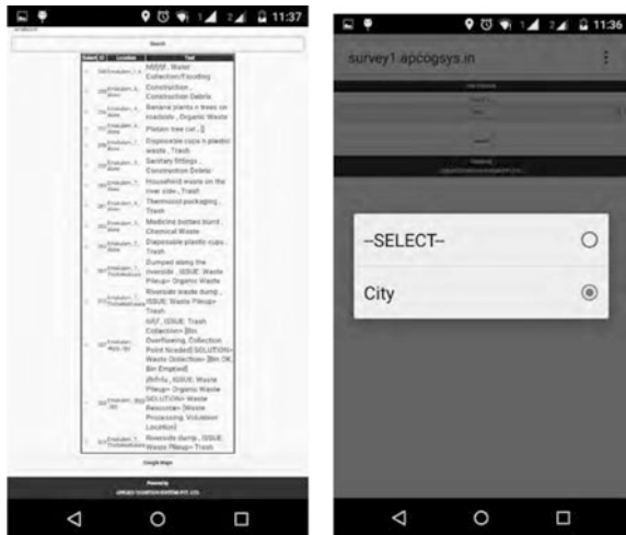
Fig. 4 Web-based tracker system using Google maps where the issue reported can be tracked by the government officials such that the solution required (for example, bin need to be emptied) can be passed on to the garbage trucks. If there are no bins located in a particular area, where there is waste piling up, the government may then need to take a different action by installing a bin or arranging for additional garbage vans that go into the area
