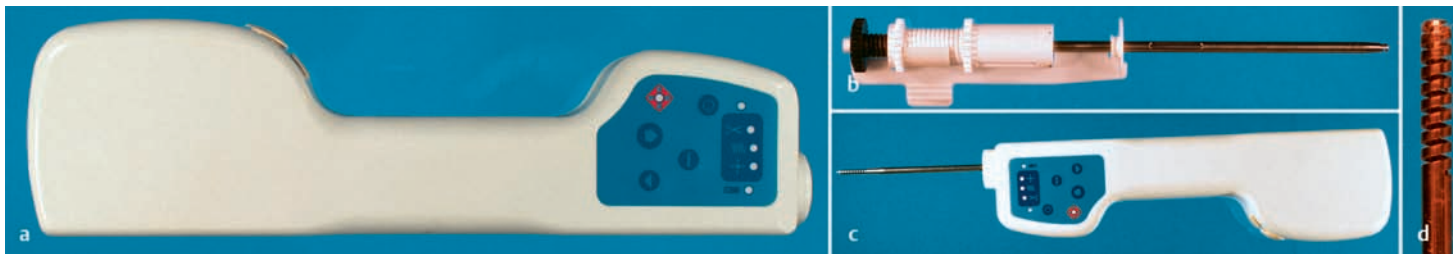
Fig. 7.27 MEDINVENTS Coramate automated large core biopsy system (Siemens, Berlin/Munich, Germany). Coramate hand-held device (a), biopsy needle (b), Coramate hand-held device with needle (c), cutting helix (d). Excision biopsy allows the collection of tissue specimens without a jet advance. A hollow metal spiral cuts in a screw-like fashion into the target tissue. The biopsy specimen is secured
