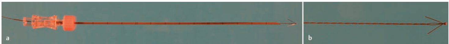
Fig. 7.48 Double hook wire localization needle (Invivo Corp., Orlando, FL). Nonretractable localization needle with hook wire (a), tip of hook wire (b). MRI-compatible: needle size: 18 and 20 gauge; needle lengths: 8, 10, 15 cm.
