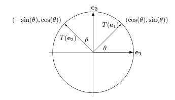
From the above, you only need to find  $T\mathbf{e}_1$  and  $T\mathbf{e}_2$ , the first being the first column of the desired matrix A and the second being the second column. From the definition of the cos, sin the coordinates of  $T(\mathbf{e}_1)$  are as shown in the picture. The coordinates of  $T(\mathbf{e}_2)$  also follow from simple trigonometry. Thus
