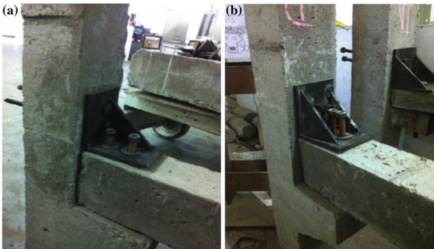
Fig. 3 Dry precast beam column connection a single stiffener and b double stiffener
