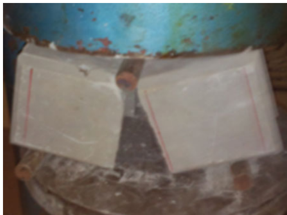
Fig. 10 Failure under flexure
