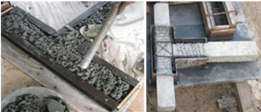
Fig. 3 Casting of control (CS) and retrofitted (NCSR) specimens
