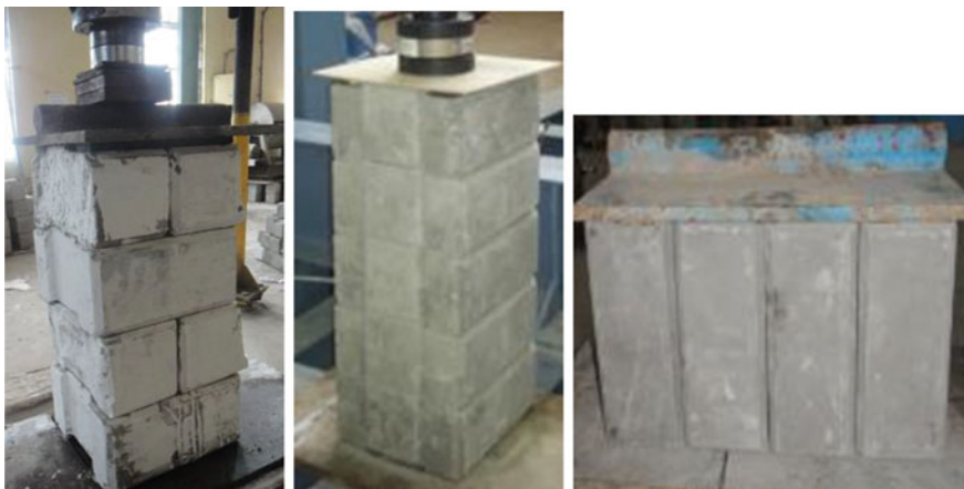
Fig. 3 Prism test setup indicating different h/t and loading direction arrangements
