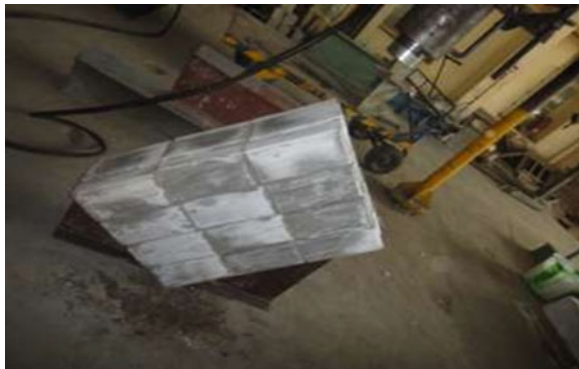
Fig. 1 Set up for diagonal compression test
