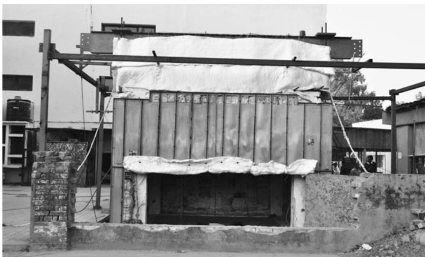
Fig. 5 View of the test frame before the fire test with ventilation window
