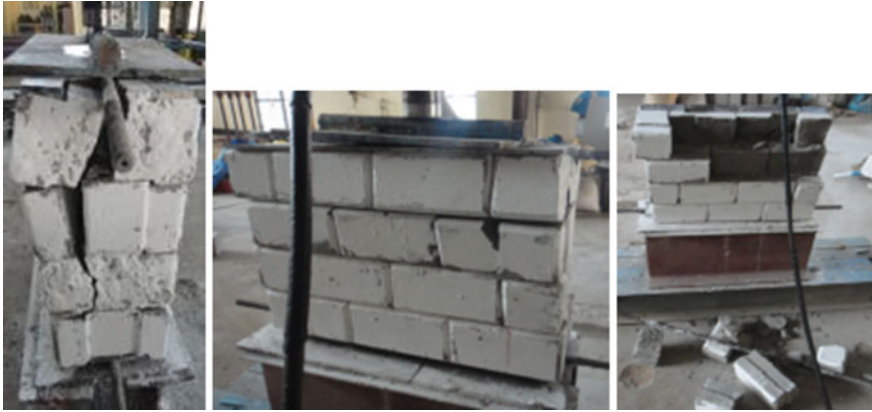
Fig. 14 Failure patterns in panels when loaded with eccentricities 0, t/6 and t/3
