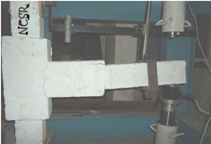
Fig. 9 Failure pattern of retrofitted specimen
