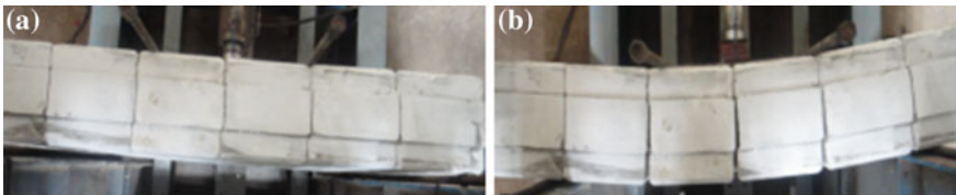
Fig. 15 a Top view of flexural loading arrangement of masonry perpendicular to bed joint and b its failed view
