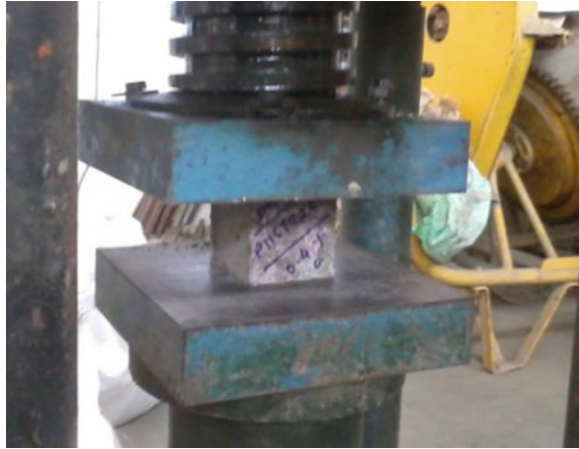
Fig. 2 Arrangement of specimen for compressive strength
