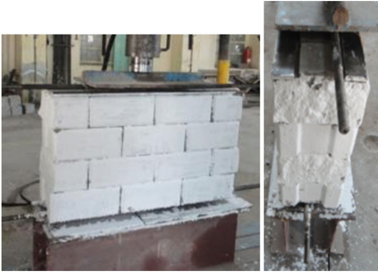
Fig. 4 Different eccentric compression test arrangements
