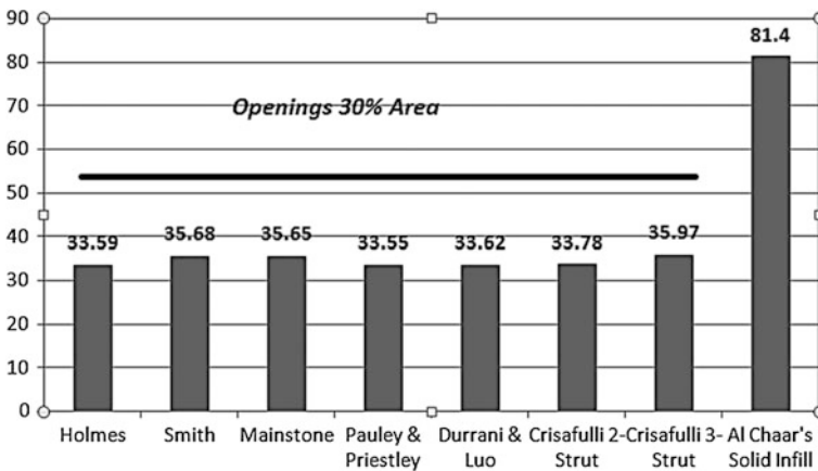
Fig. 4 Peak load variation for Al-Chaar's model with change in modeling
