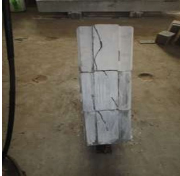
Fig. 2 Crack pattern due to diagonal compression test
