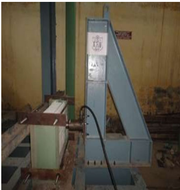
Fig. 3 Out-of-plane testing on GPC wall
