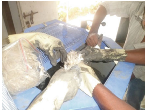
Fig. 5 Mixing of biofibres while casting
