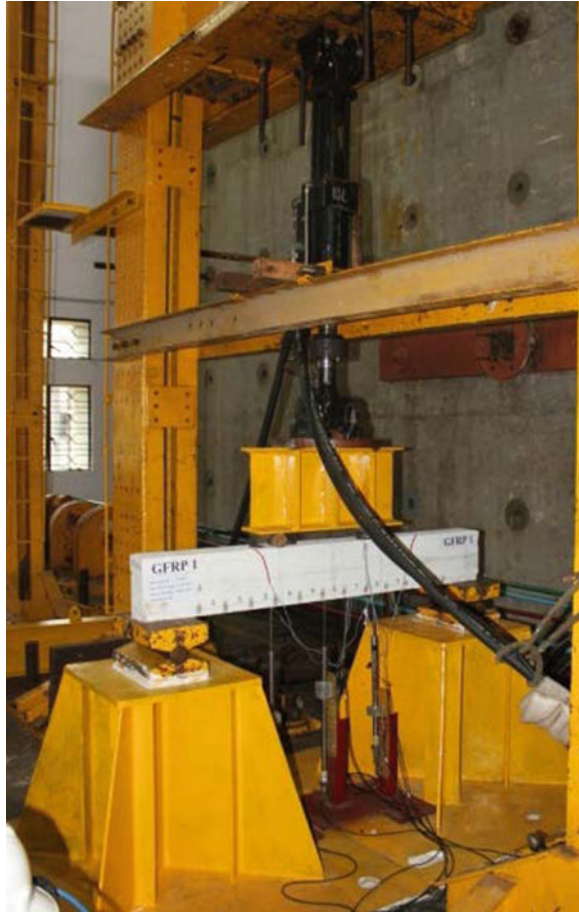
Fig. 5 Experimental test set up for static/fatigue tests
