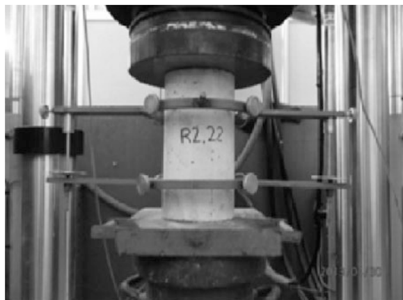
Fig. 1 Test set up for axial compression test to determine compressive stress and stress-strain curve
