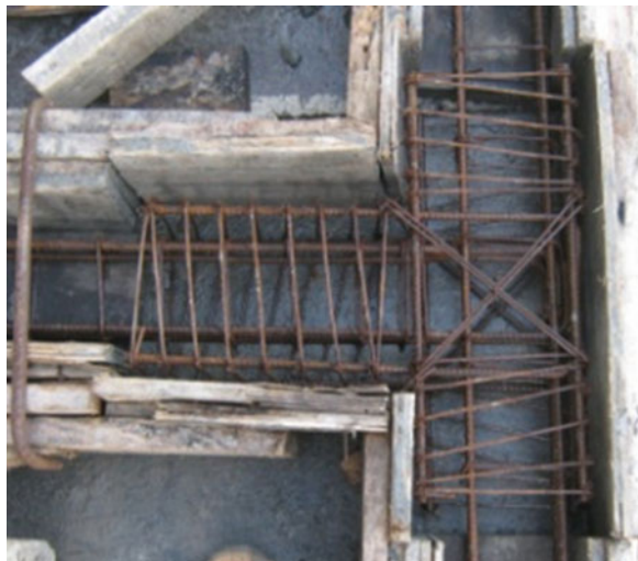
Fig. 3 Casting of control (CS) and retrofitted (NCSR) specimens
