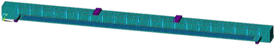
Fig. 3 Finite element modeling showing finite elements and mesh density
