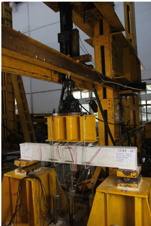
Fig. 7 Fatigue test set-up for concrete beams reinforced with GFRP bars
