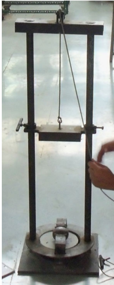
Fig. 3 Arrangement of specimen for impact test
