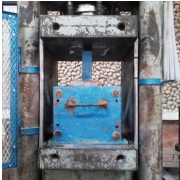
Fig. 6 Photograph of mechanical press by compression testing machine
