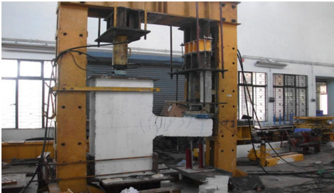
Fig. 8 Experimental test setup for monotonic test
