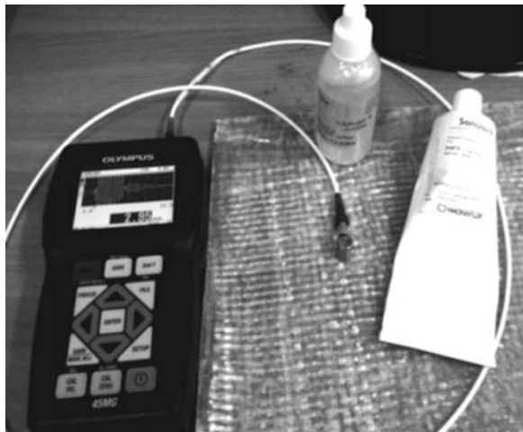
Fig. 4 Ultrasonic sound velocity measurement set-up
