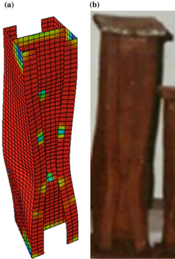
Fig. 2 Failure of deformed shape. a FEA. b Experimental
