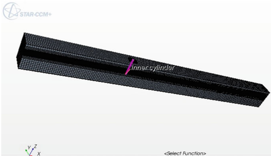
Fig. 4 Domain of inner cylinder generated with volumetric control
