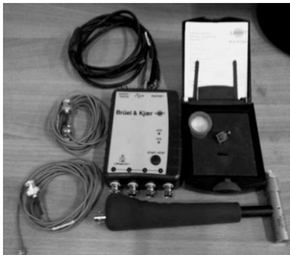
Fig. 5 B&K modal analysis instruments
