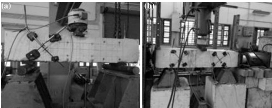
Fig. 4 Test set-ups. a Set-up for testing under lateral load only. b Set-up for testing under simultaneous lateral and axial loads
