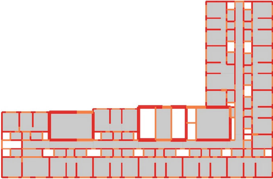
Fig. 4 Model II (modular wall slab construction type)
