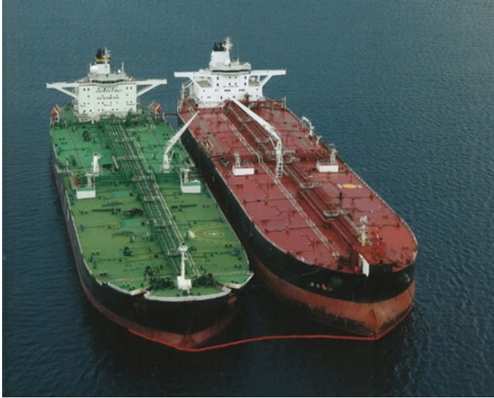
Fig. 8.1 A typical STS transfer of oil cargo operation (Source: OCIMF 2013)
