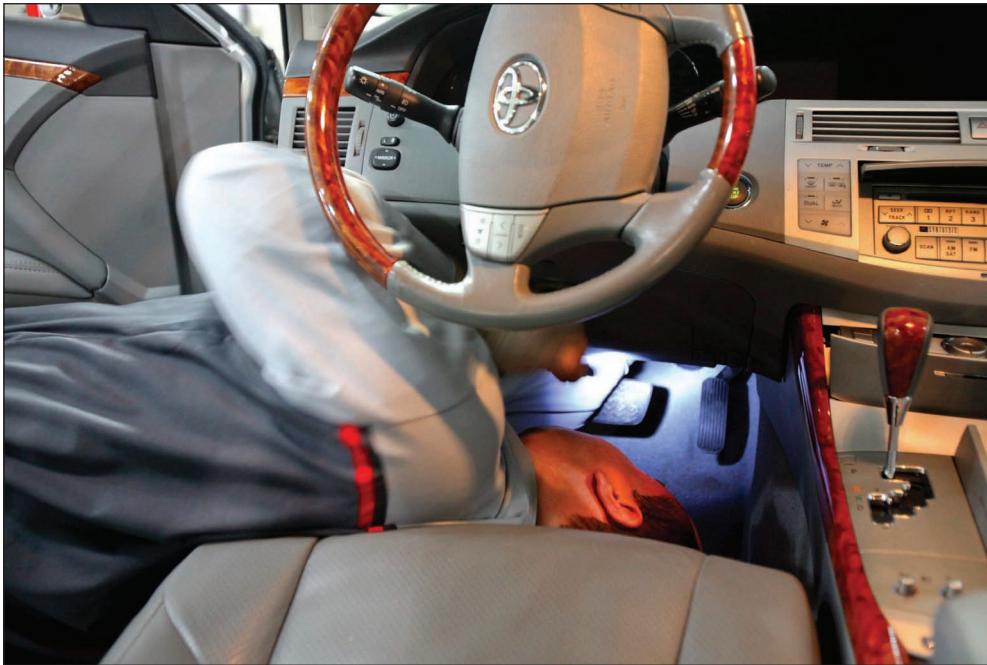
A Toyota technician prepares to remove the accelerator assembly in a recalled Toyota Avalon.
