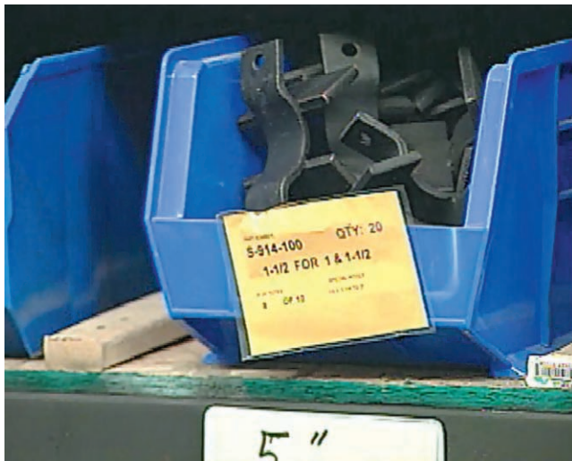
At TriState Industries, a kanban system is in effect to move work through the production system. Shown here, a kanban card provides the authorization to move or work on parts.
