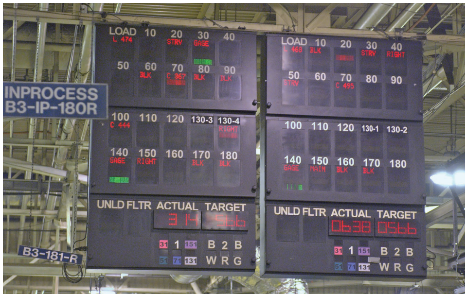
The Andon board in the GM Powertrain Engine facility is a visual communication tool. It advises employees of the real-time status of each machine within the manufacturing lines, enabling the production system to be run more effectively.
