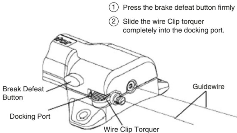
FIGURE I.4 WireClip torquer docking port (Image provided courtesy of Boston Scientific. © 2017 Boston Scientific Corporation or its affiliates. All rights reserved)
