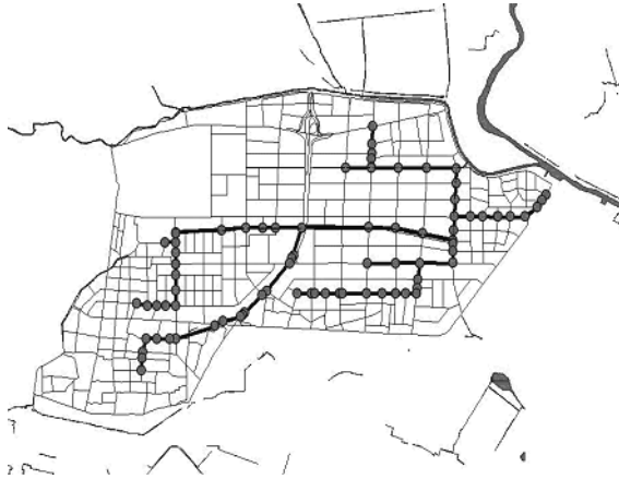
Fig. 4. Drainage network of 2000 mm or more.
