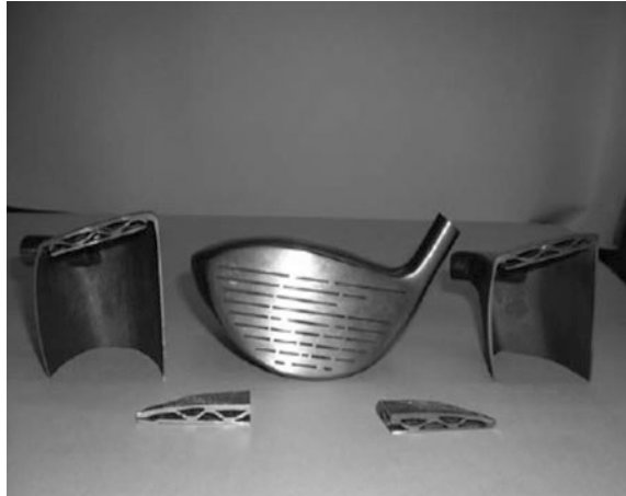
Fig. 4.6 Components of golf club made from nanostructured Ti–6Al–4V alloy. The figure is reproduced from [38] with permission of the publisher Institute of Problems of Mechanical Engineering RAMS
