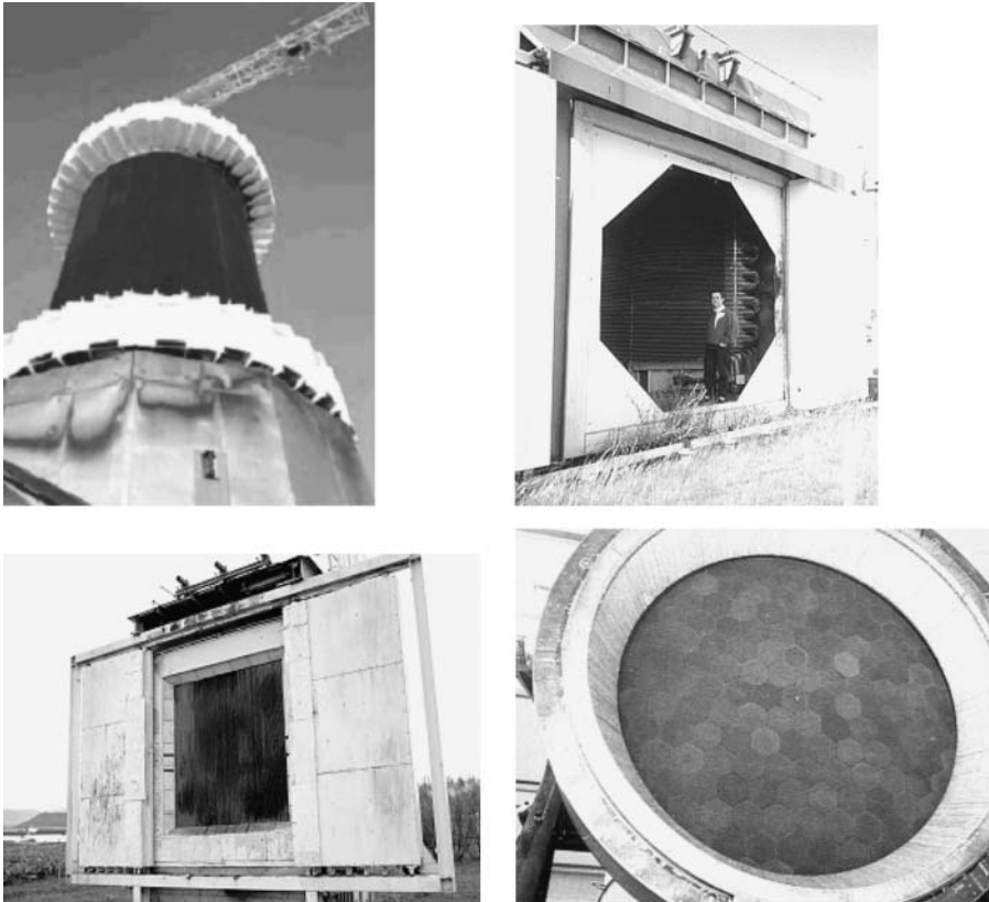
FIGURE 19.49 Different configurations of solar receivers. From left to right and top to bottom: (a) external tubular cylindrical, (b) cavity tubular, (c) billboard tubular, and (d) volumetric.
