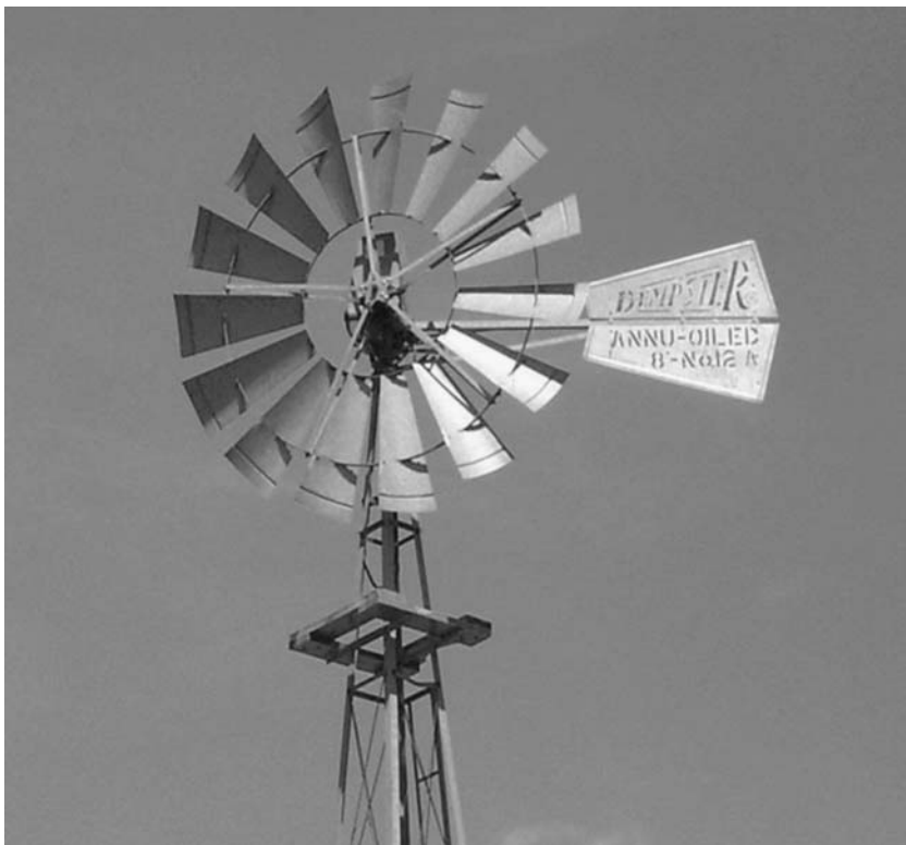
FIGURE 21.2 Typical American multiblade windmill. (Courtesy of Nolan Clark, U.S. Department of Agriculture).
