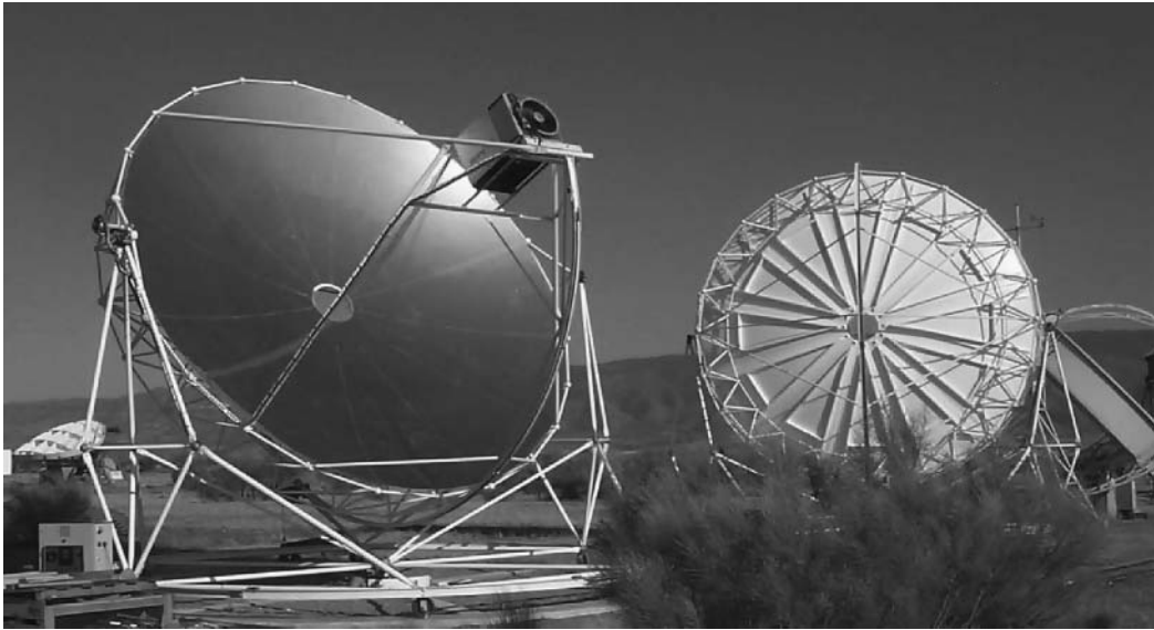
FIGURE 19.70 Example of segmented parabolic concentrators. Rear and front view of two EuroDish prototype tested at the Plataforma Solar de Almería, Spain.
