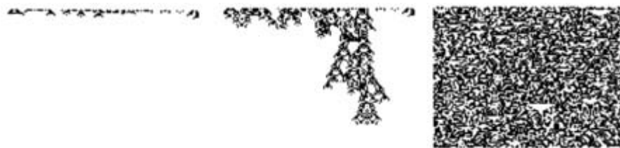
Figure 6.2 Evolution of one-dimensional cellular automata. Each horizontal line represents one automaton state. Successive time steps are shown as successive horizontal lines. Sites with value 1 are represented by black squares; sites with value 0 by white squares. One example each for an automaton of class 1 (left), class 4 (middle), and class 3 (right) is given.
