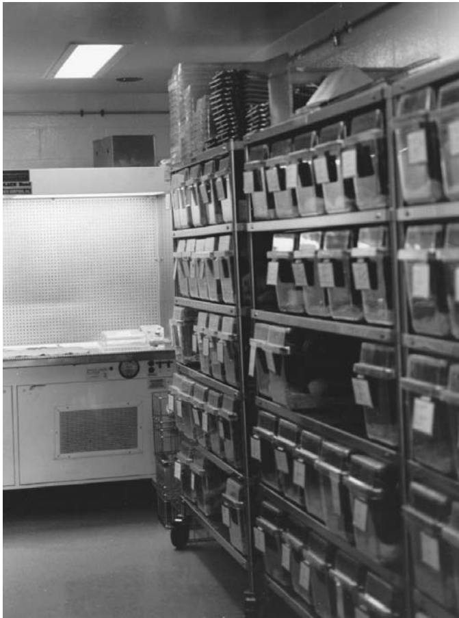
Fig. 7. Typical secondary enclosure setup. The primary enclosures in this barrier facility are placed onto racks with cage changes occurring in the hood at the back of the room.
