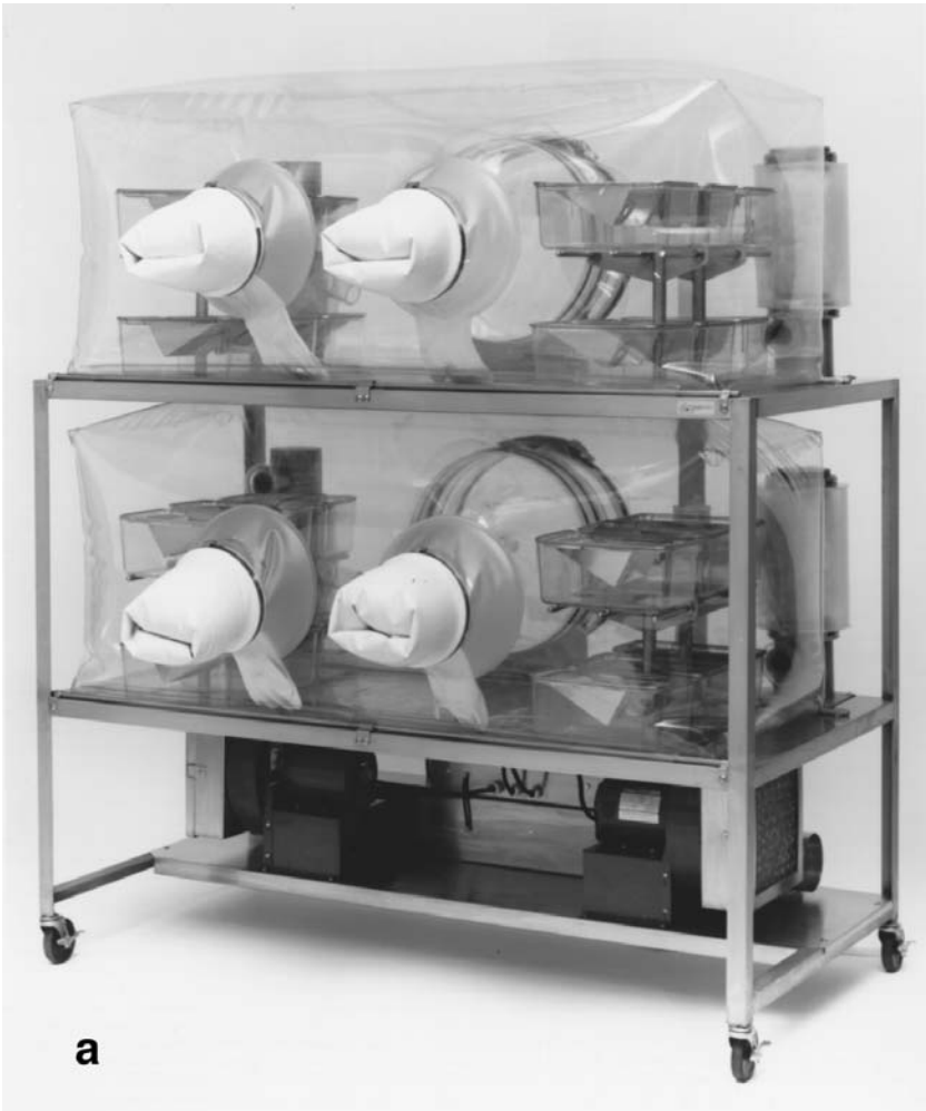
Fig. 9. (a) The front view of a flexible film isolator. There is no need for microisolator tops for the cages as animal manipulations are performed by individuals using the attached gloves. (b) The back view of a flexible film isolator. The unit on the bottom shelf is responsible for moving HEPA (High Efficiency Particulate Arrestance) filtered air in and out of the unit. The two large circular ports in the top two shelves are used to move materials in and out of the isolator. (Photo courtesy Karen Holland, Class Biologically Clean, Ltd., 2901 Latham, Madison, WI 53173.)
