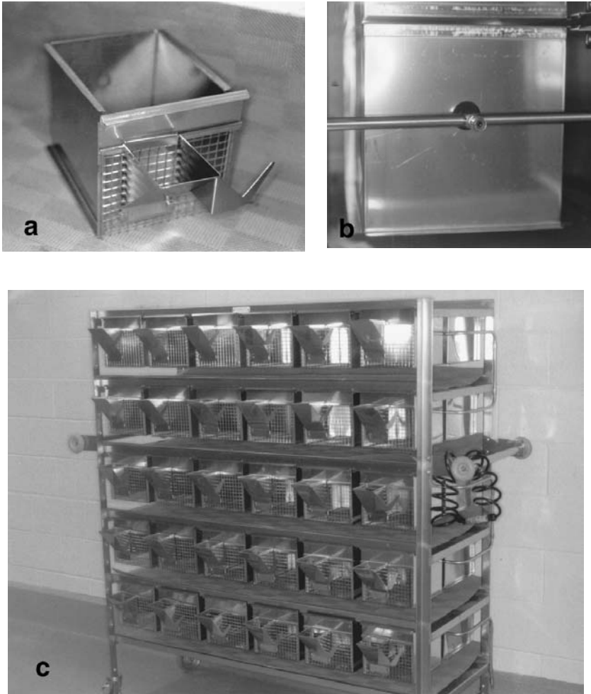
Fig. 3. The stainless steel primary enclosure (a) has a V-shaped notch to hold the water bottle and a feed bin immediately to the left; (b) the circular hole at the rear may be used for entry of an automatic watering spout; (c) the flanges at the top of the enclosure permit the cage to slide in and out of the rack.
