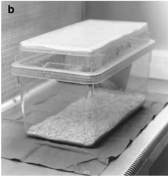
Fig. 5. The addition of the microisolator top prevents contamination from the micro- and macroenvironment. (a) side view, (b) front view.
