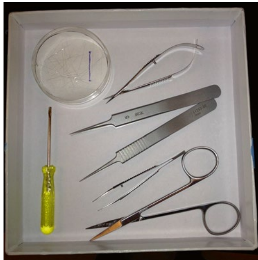
Fig. 1 Tools to dissect and mount the vessels into the wire myograph. The small petri dish contains 2-cm-long wires. The blue mark on the petri dish marks a length of 2 cm to facilitate cutting the wires
