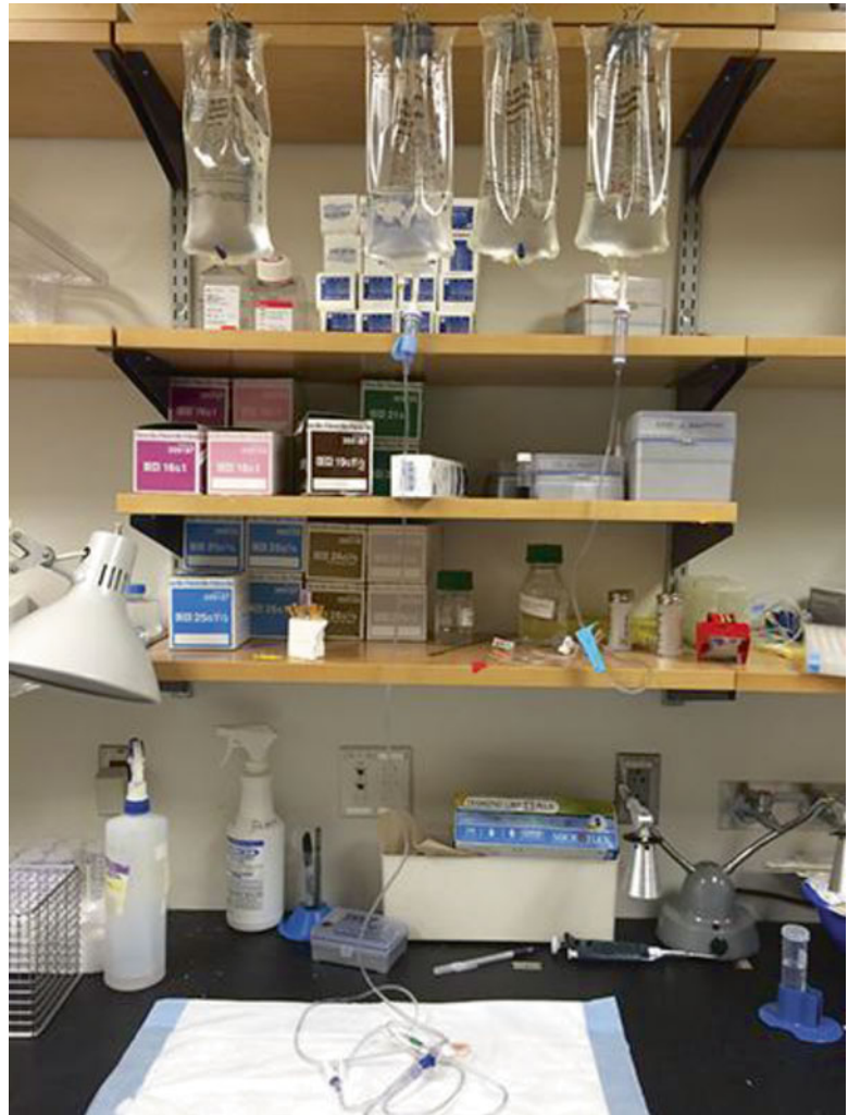
Fig. 1 Gravity flow apparatus for vascular perfusion. Perfusant is suspended at a height of 60 cm above the mice to be perfused so as to maintain a pressure of 60–100 mmHg and a flow rate of 1–3 ml/min
