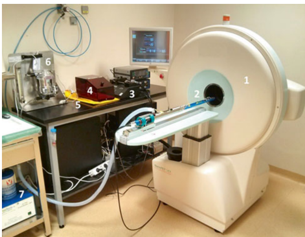
Fig. 1 PET/CT scanner and different equipment needed for anesthesia, injection of CT contrast agent, and temperature control
