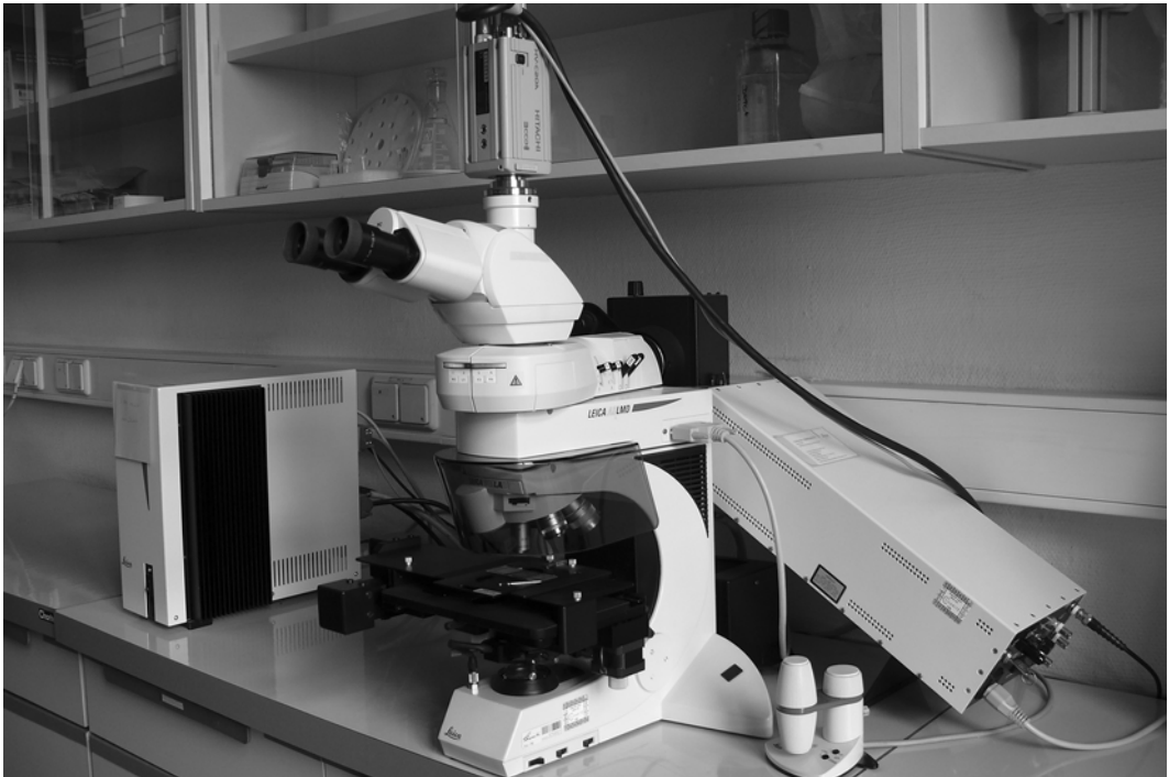
Fig. 2 Laser Microdissection System Leica DMLA. The Leica CTR MIC electronics box is placed slightly distant from the microscope ( left side ). To the right , you see the Smartmove control in front and the laser cartridge behind. Pictures are transmitted from the camera ( on top ) to a computer providing the LMD software
