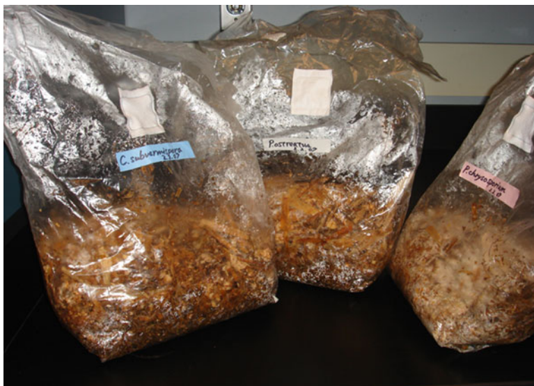
Fig. 19.2 Biological pretreatment of corn stover (particle size >1 mm) with white rot fungi
