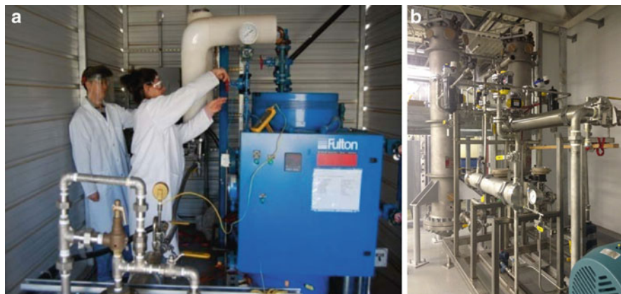
Fig. 19.3 (a) Steam Gun at UC-Riverside and (b) AFEX Pretreatment Reactor at MBI (Courtesy: http://www.cert.ucr.edu/Cellulosic%20Biomass.pdf and http://www.mbi.org/technologies-3/afex/ )
