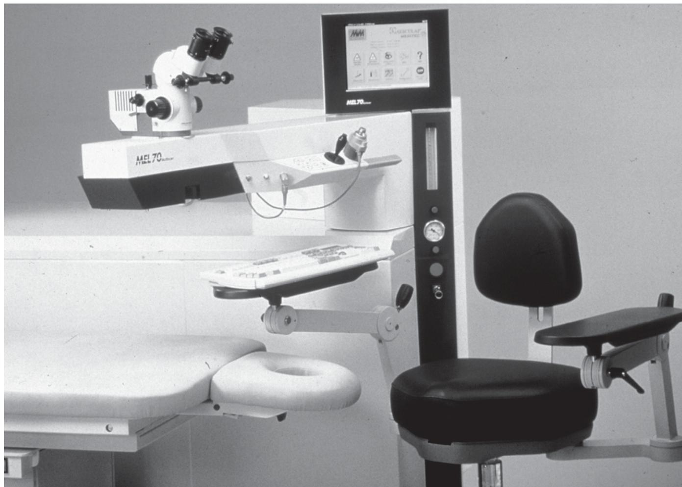
**Figure 89.5.** The Aesculap-Meditec MEL-80 laser (Aesculap-Meditec, Jena, Germany) has a small flying spot that scans across the cornea for myopic, hyperopic, and astigmatic treatments. (Courtesy of Aesculap-Meditec, Jena, Germany.)
