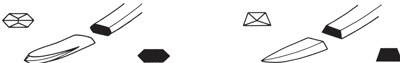
**Figure 37.3.** Concave spatula (CS) design of Ethicon surgical needle. (Courtesy of Ethicon, Inc, Somerville, NJ.)
