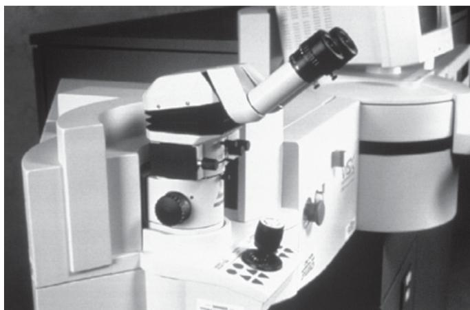
**Figure 89.3.** The control panel of the VISX Star laser (VISX, Santa Clara, CA) includes a joystick for moving the patient's bed, a Leica Wild microscope (Leica, Inc., Allendale, NJ) and controls for ring and oblique lighting. (Courtesy of VISX, Inc., Santa Clara, CA.)
