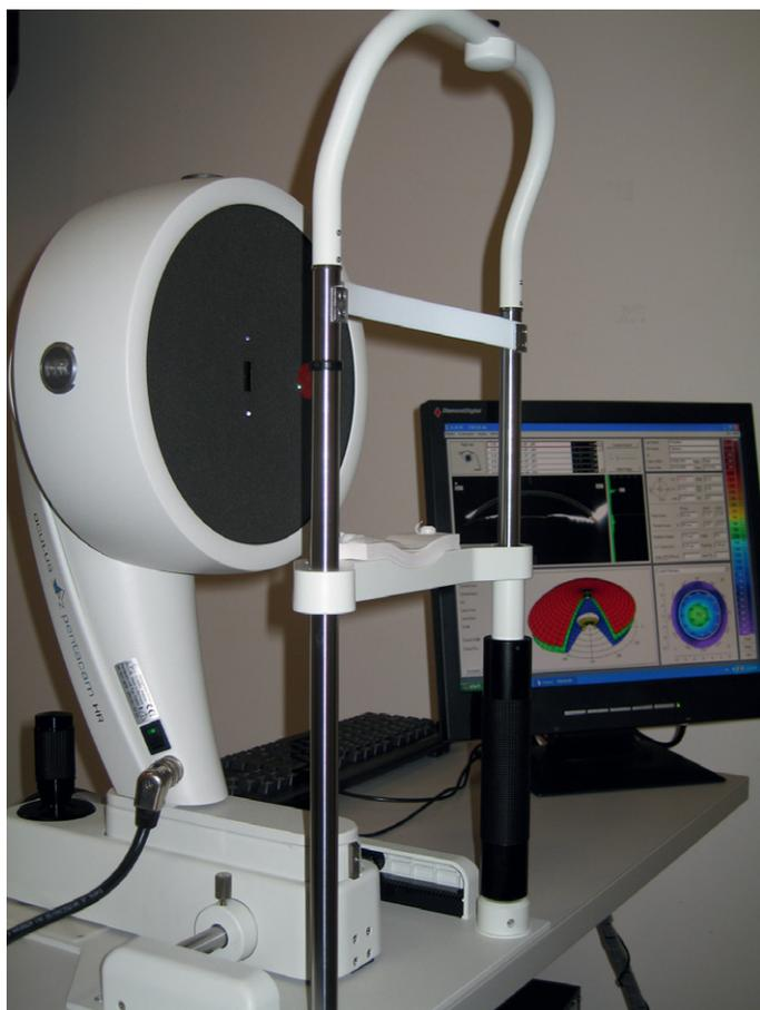
**Figure 10.5.** Oculus Pentacam Scheimpflug tomography device.
