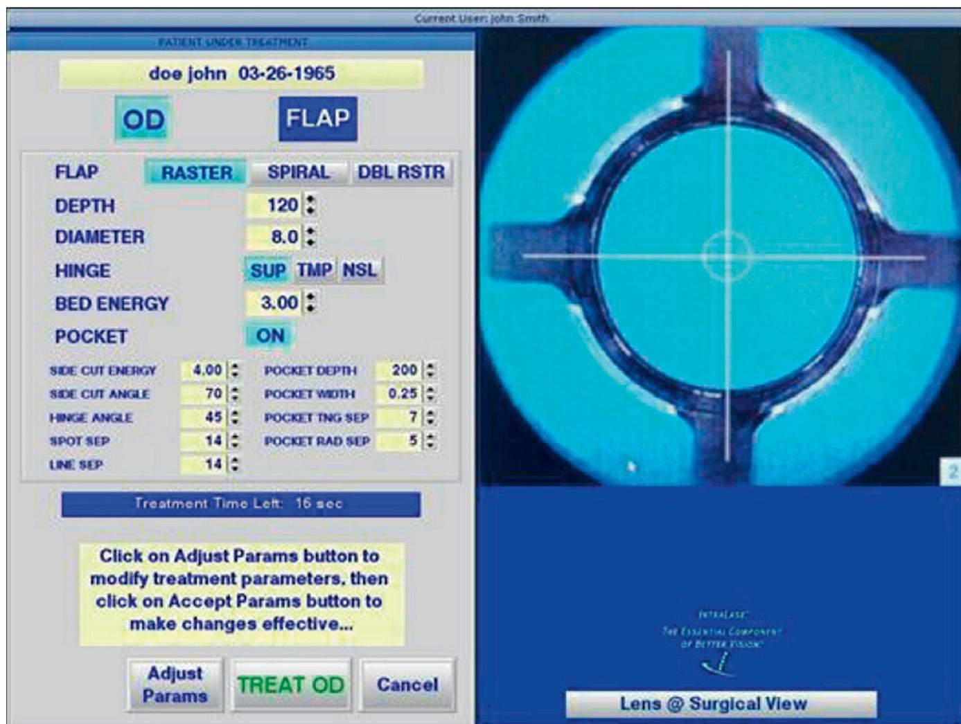
Figure 95.7. Graphical user interface of IntraLase® FS laser. Based on photograph courtesy of IntraLase®.
