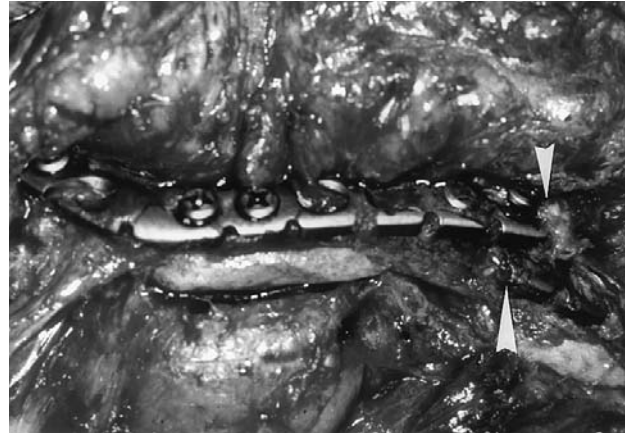
FIGURE 27.6 Clinical site of a plate fracture in a case of alloplastic repair (arrows).
