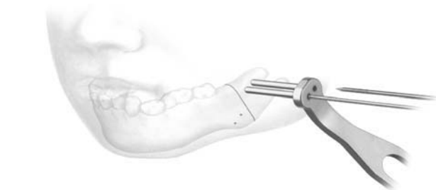
FIGURE A1.16 Insertion of screws via trocar. (Courtesy of Synthes Maxillofacial, Paoli, PA)
