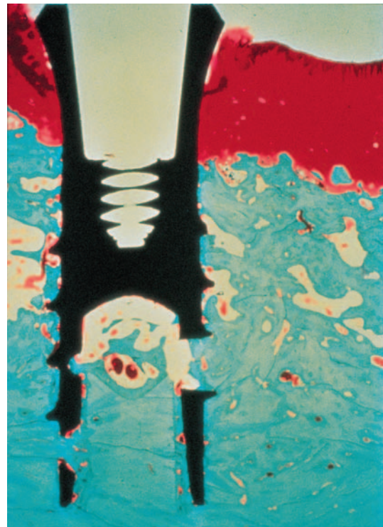
FIGURE 15.7 Micrograph demonstrating direct bone-to-implant contact (osseointegration) to TPS surface (experimental sample from primate).
