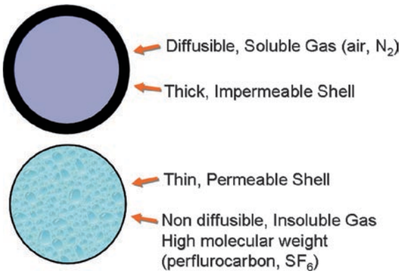
Fig. 30.1 In order to survive transpulmonary passage and persist in the circulation, the gas within contrast agents must be prevented from diffusing into blood. This is achieved either by using a thick, impermeable shell or by using a high molecular weight, insoluble gas
