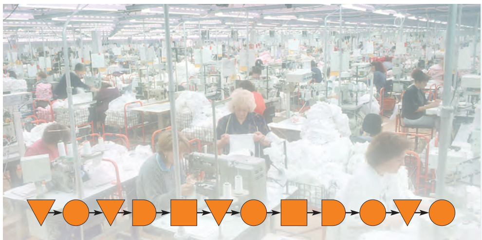
Figure 4.6 A batch process in a garment manufacturer together with an illustrative process map
