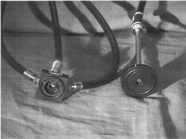
Figure 1. The two fibers-probe configuration used in connection with the spectrum analyzer. Left dark hemisphere probe; right drilled cylinder probe.
