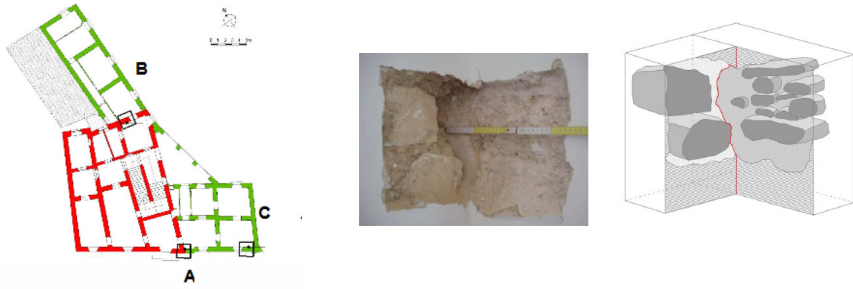
Figure 13: Sardi Palace in Palizze street: ■ original parts; ■ parts added in 19 th century. Figure 14: Study of wall interlocking at corner A of fig. 13.
