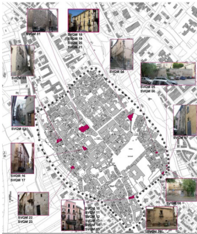
Figure 3: Recognition of building facades without plaster for masonry qualification.
