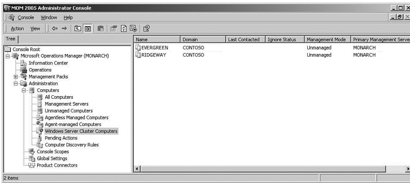
FIGURE 15.22 Windows Server Cluster Computers in the Administrator console.
